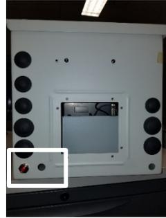
13. Remove the black protective plug from the antenna hole in the enclosure.
