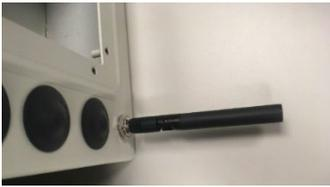
22. Attach the terminator plug to the board ANT-2 (J43) connector (see number 1, below).
