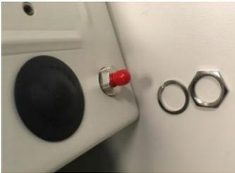
15. Ensure the gasket that was installed in step 11 is between the surge-protector and the enclosure (on the inside of the enclosure).
