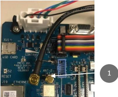
The Wi-Fi antenna installation is complete.
