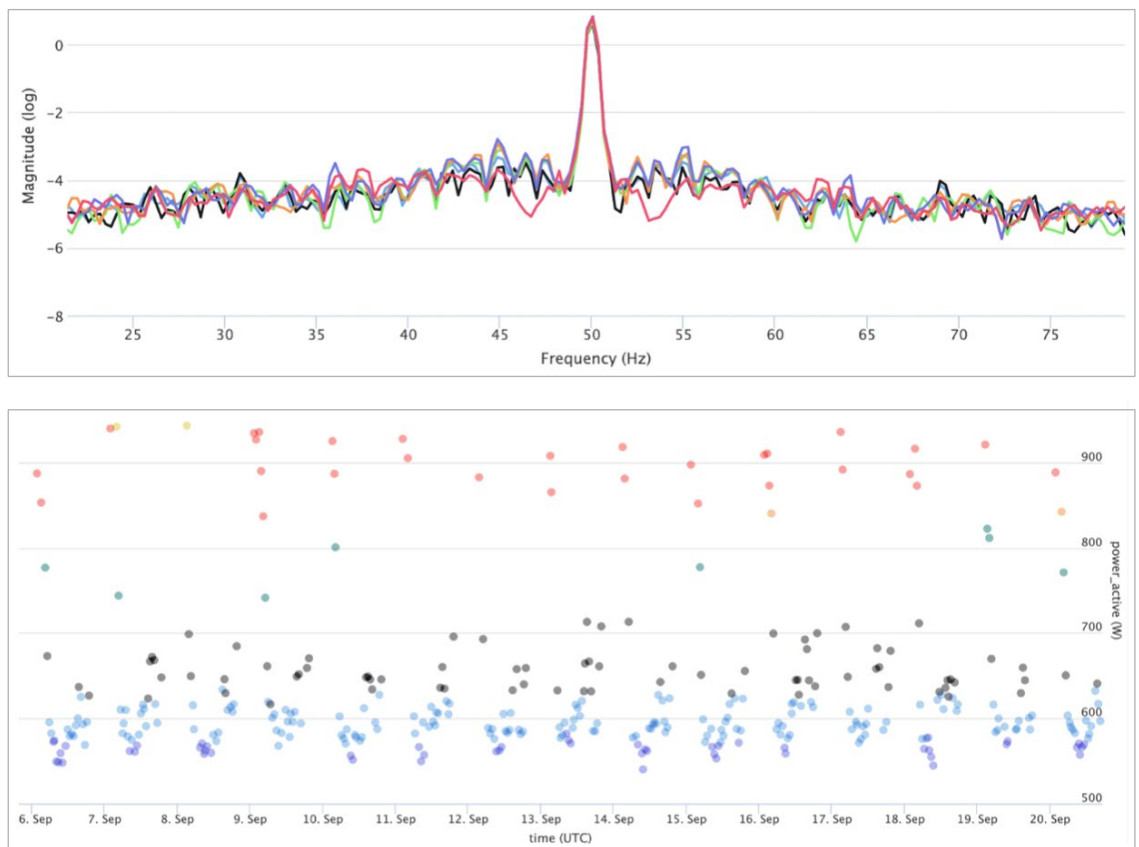
Figure 10. Each color represents this machine's frequency signature (top) at a different load (active power, bottom). Note how much the signatures vary – if we didn't know they represented different situations, we would either flag nonexistent damage (because behavior has visibly changed) or miss real damage (because our definition of "healthy behavior" is too broad). Only systems that measure current + voltage can automatically eliminate these risks.
