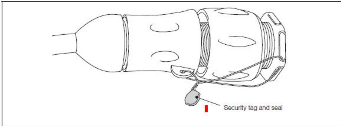
**Figure 3 Transmitter Sealing**
