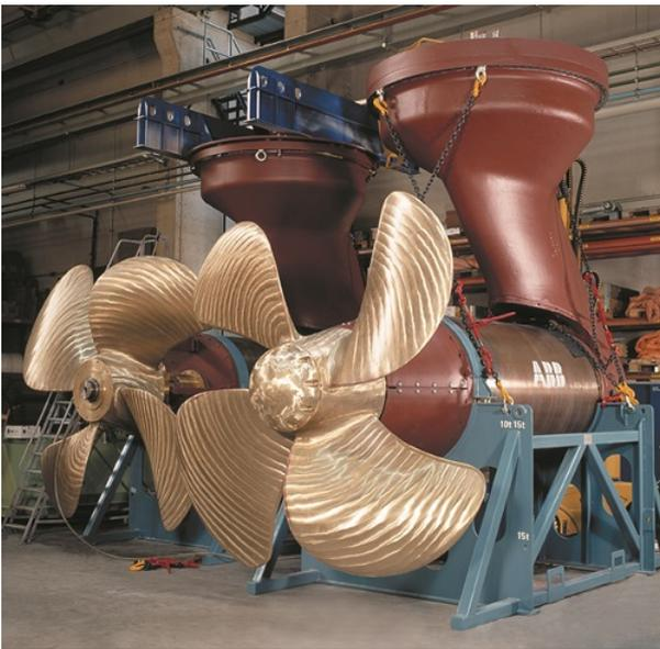
ABB's new Azipod D will complement the Azipod C thruster, which since its introduction more than a decade ago has been installed on more than three dozen vessels
