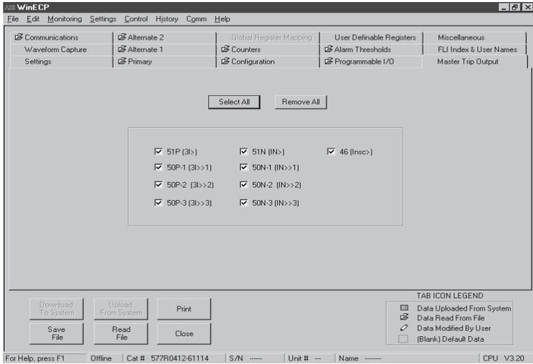
Figure 6-2. Master Trip Contact Programming Screen
