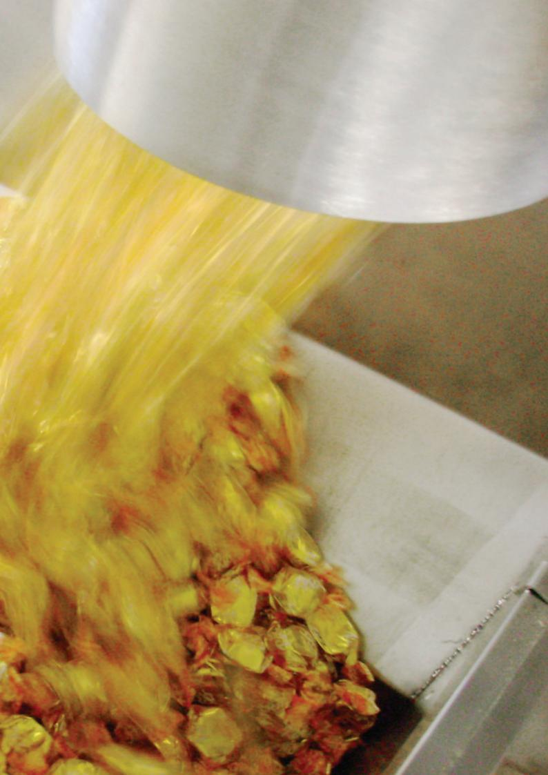
HD cameras are located at the entry to each packing plant distribution system, this defines / distributes the correct unit to the correct hopper lane. Across both plants there are a total of 35 lanes with intelligent accumulation, giving sufficient buffer capacity prior to the automatic tipping machines. Developed specifically for the project by CKF, the tipping machines deliver units into the feed hoppers upon demand.
