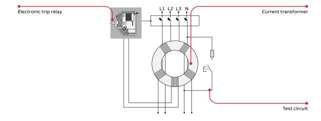
Figure 3: inside a GFEP device
