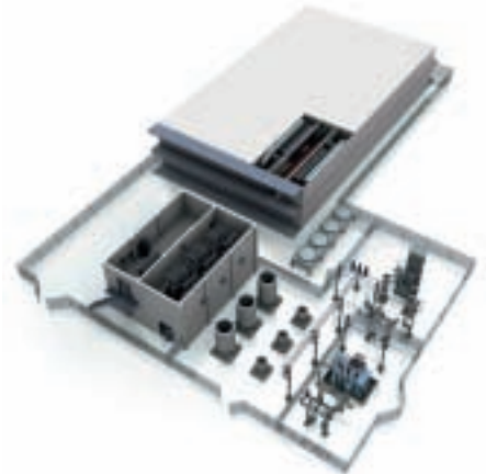
9 An impression of an SVC Light® with Energy Storage installation
