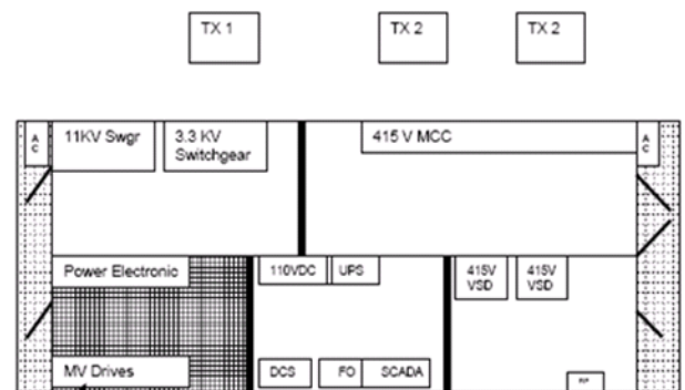
Isolate MV drives and Power Electronic Shield from rest of system. Faraday Cage
