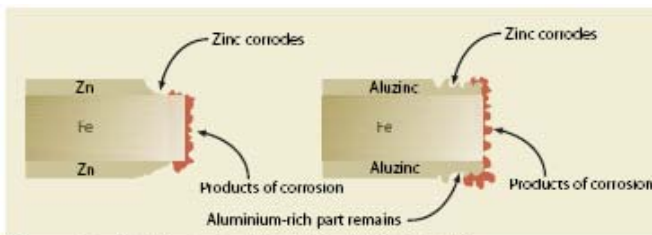
Edge corrosion of hot-dip galvanized steel (left) and of Aluzinc (right).
