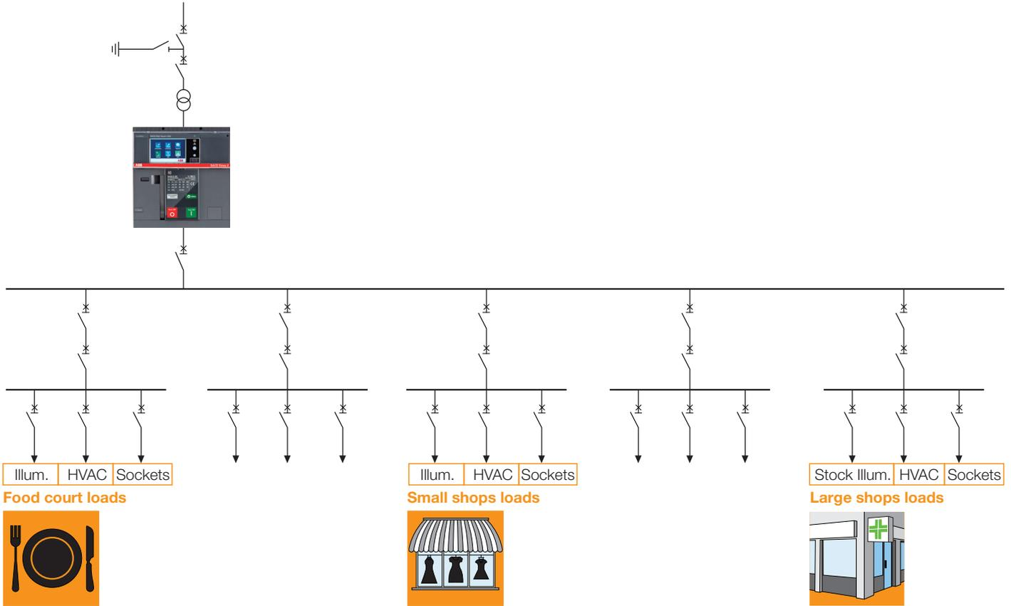
A commercial installation is reported here above: some loads (like HVAC) can be disconnected for a certain amount of time without compromising the plant functions.
