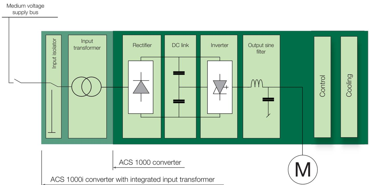
The ACS 1000 drives family's well proven three-level inverter, without series or parallel connected power semiconductors, is one of the least complex, most robust and efficient drive topologies.
