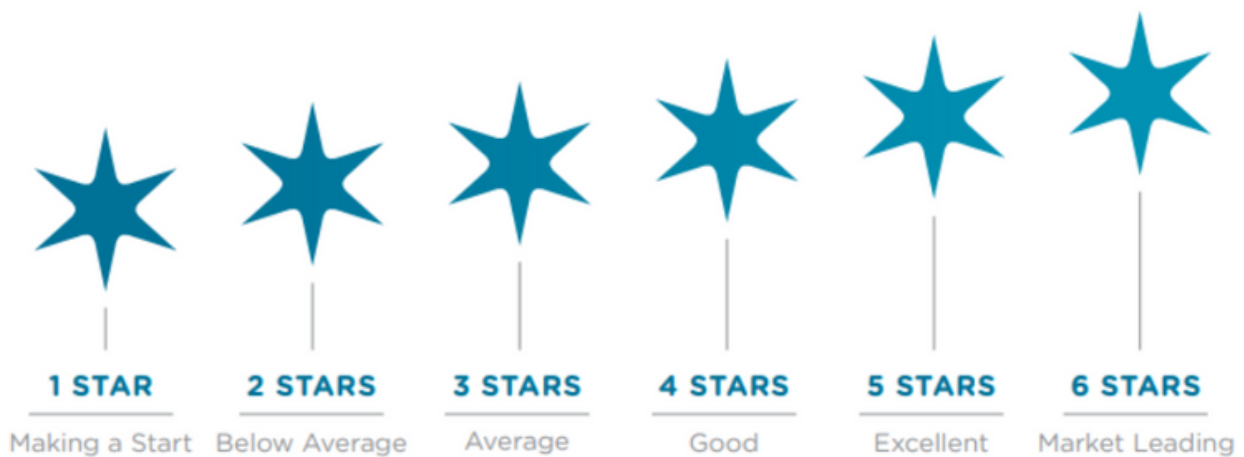
Figure 1: NABERS is a simple, reliable sustainability rating for the built environment. This rating provides a rating from one to six stars for buildings efficiency. This helps building owners to understand their building’s performance versus other similar buildings, providing a benchmark for progress. The NABERS rating is valid for 12 months.
