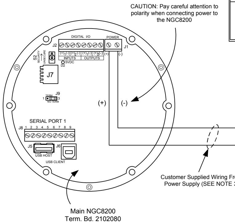
3. Wire size is a function of the distance between the NGC and the DC Power Supply. With the condition of a single heater used on both NGCs, use 8 Amps as the maximum current draw to calculate an adequate wire size so that the voltage measured at the NGC's Power I/O terminal is a minimum of 10.5 Volts.
