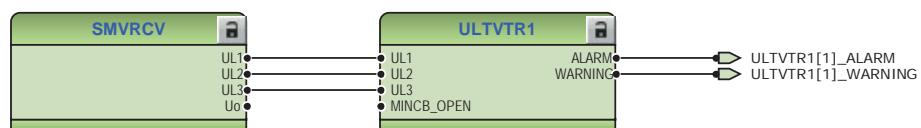
Figure 83: Connection of SMVRCV to ULTVTR1 in Application Configuration
