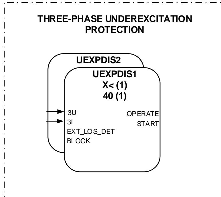
*Figure 47: Three-phase underexcitation protection*
