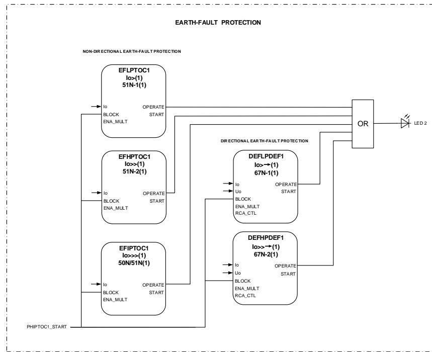
Figure 61: Earth-fault protection
