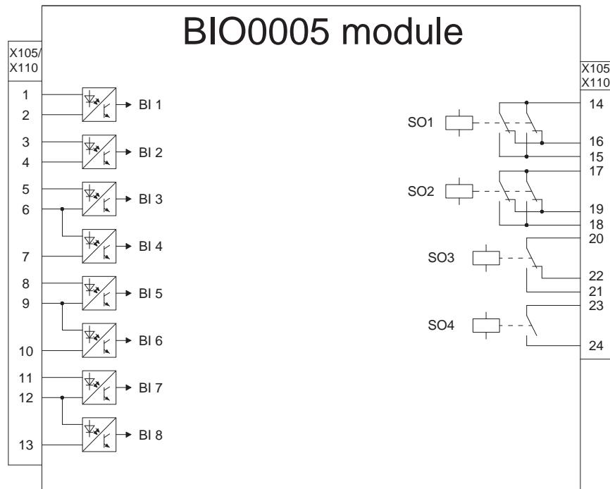
Figure 16: Optional BIO0005 module (slot X105)
