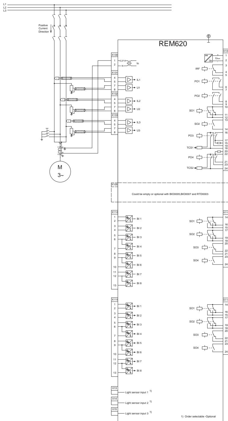
Figure 14: Connection diagram for the configuration with SIM0002 module
