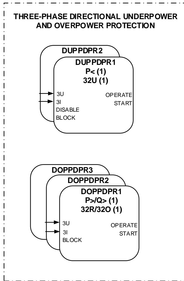
Figure 80: Three-phase directional underpower and overpower protection function
