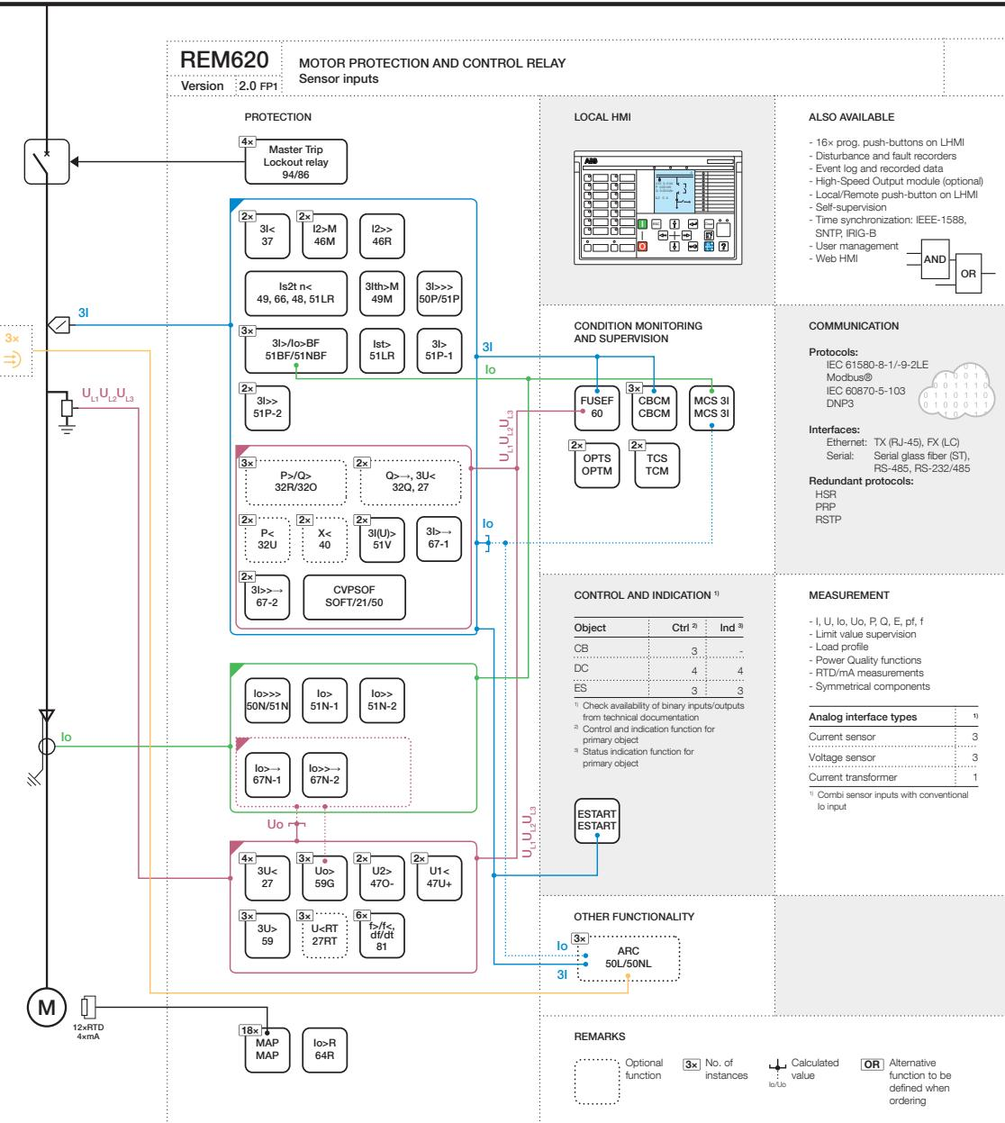
Figure 57: Functionality overview of default configuration with sensor inputs
