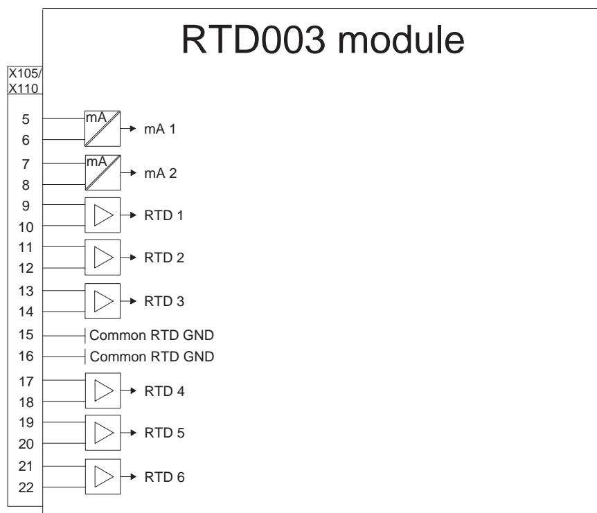
Figure 18: Optional RTD0003 module (slot X105)
