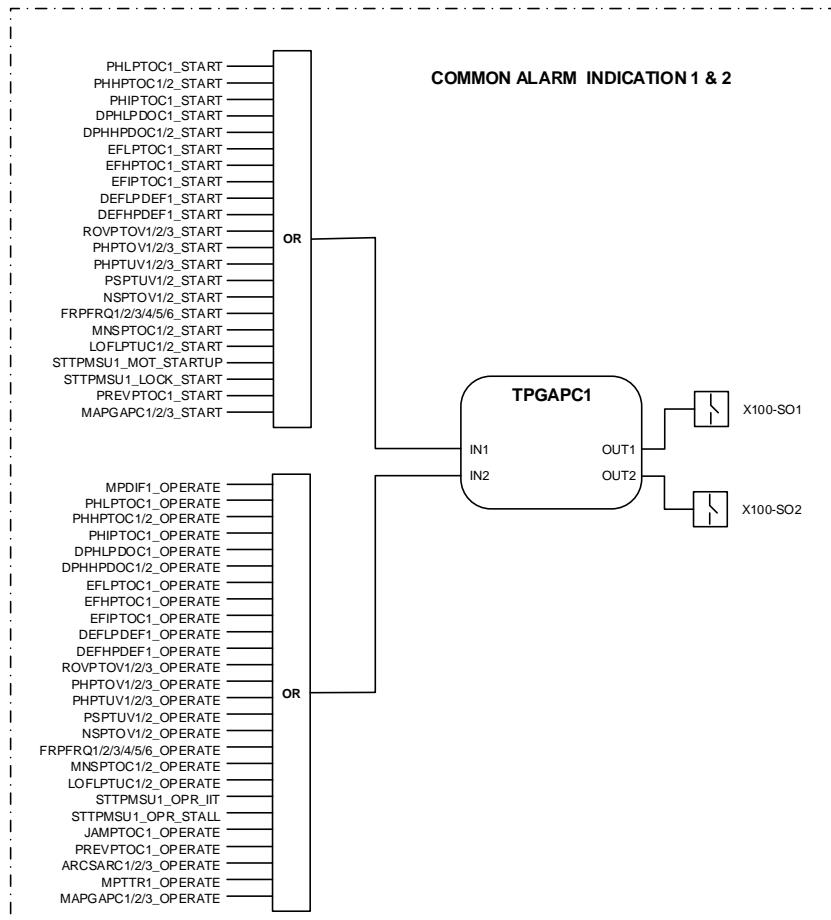
Figure 40: Common alarm indication
