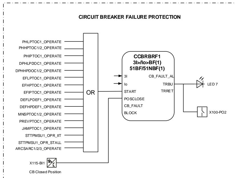
*Figure 69: Circuit breaker failure protection*
