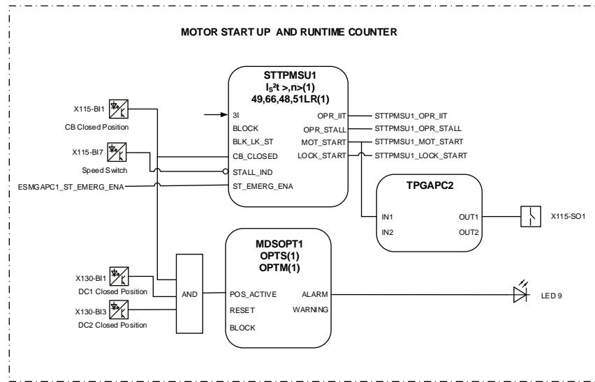
Figure 29: Motor startup supervision
