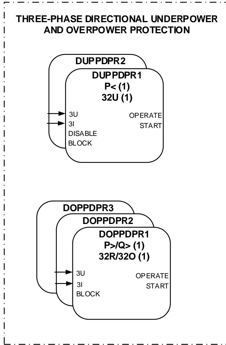
Figure 46: Three-phase directional underpower and overpower protection function
