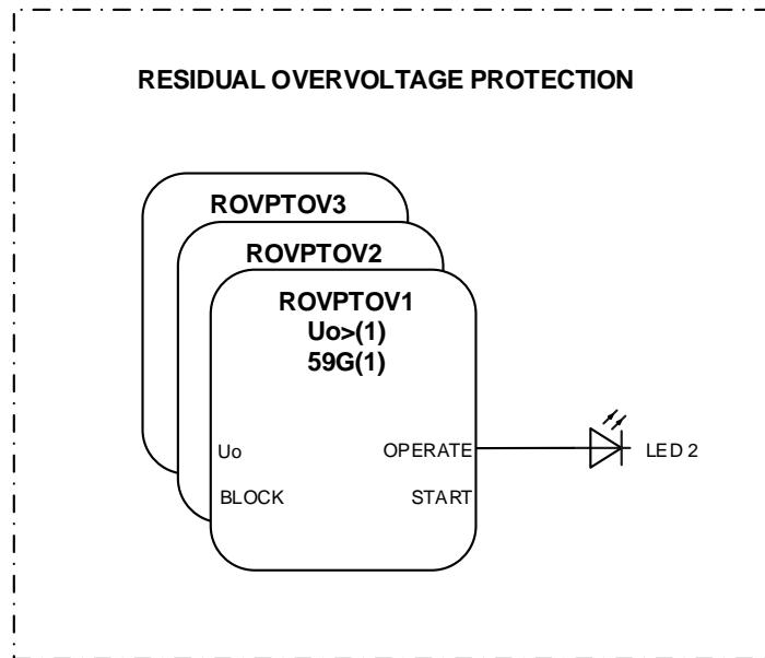
Figure 64: Residual overvoltage protection
