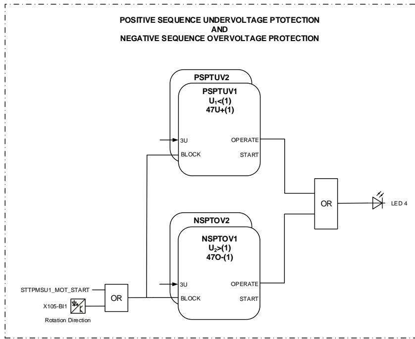
Figure 26: Positive-sequence undervoltage and negative-sequence overvoltage protection
