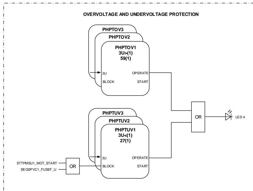
*Figure 25: Overvoltage and undervoltage protection*
