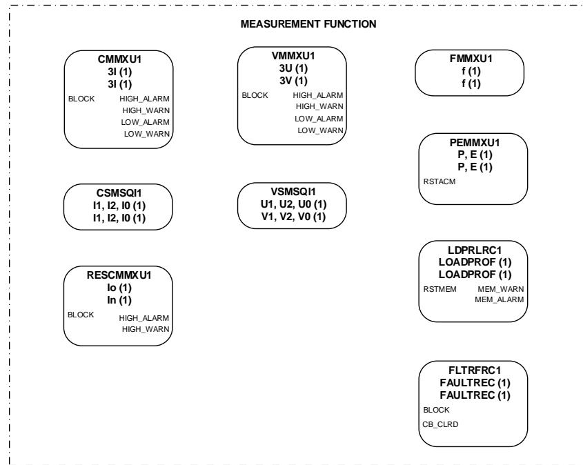
Figure 77: Measurement function
