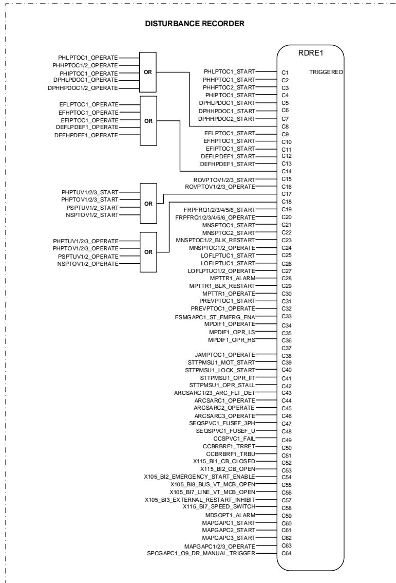
Figure 35: Disturbance recorder
