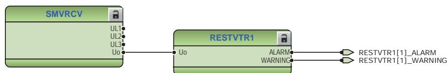
Figure 51: Connection of SMVRCV to RESTVTR1 in Application Configuration
