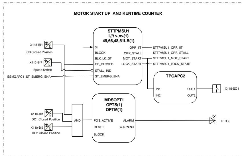
*Figure 66: Motor start-up supervision*
