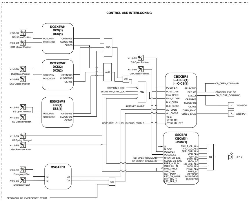
Figure 39: Circuit breaker control and interlocking
