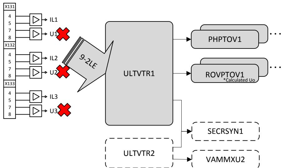
Figure 84: ULTVTR1 uses three phase voltages from received IEC 61850-9-2 LE sample value
