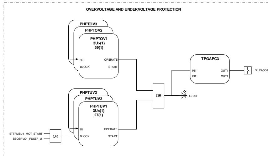
*Figure 62: Overvoltage and undervoltage protection*
