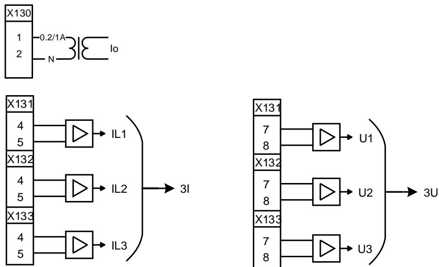
Figure 58: Physical analog channels in default configuration B
