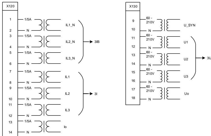
Figure 20: Physical analog channels in default configuration A
