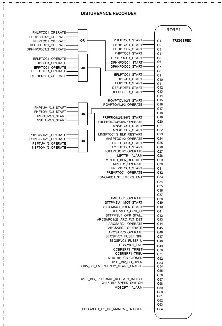
Figure 71: Disturbance recorder
