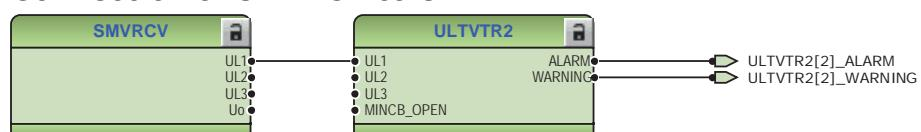
Figure 55: Connection of SMVRCV to ULTVTR2 in Application Configuration
