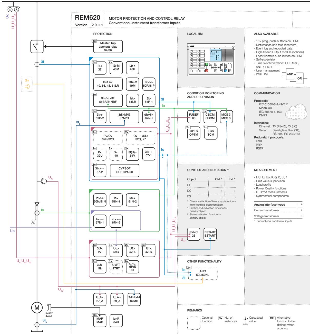
Figure 19: Functionality overview of default configuration with conventional instrument transformer inputs
