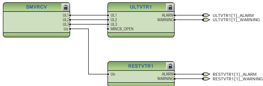
Figure 53: Connection of SMVRCV to both ULTVTR1 and RESTVTR1 in Application Configuration
