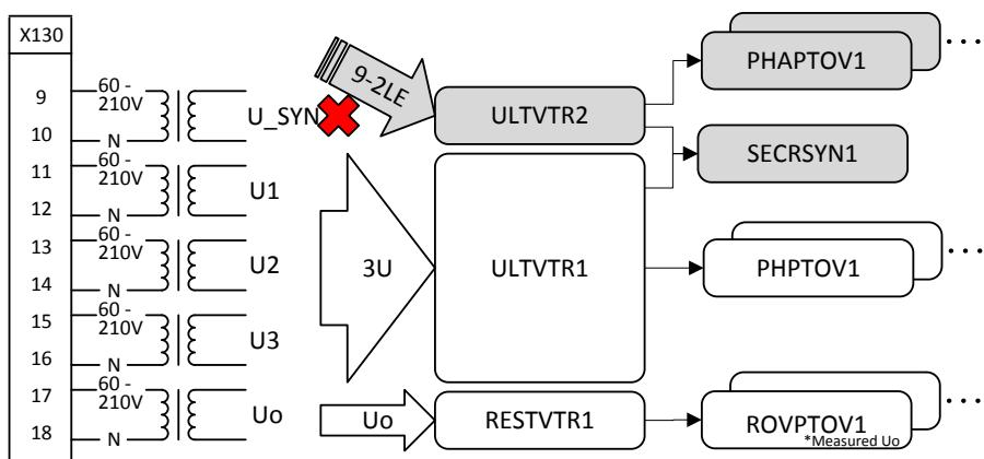
Figure 56: ULTVTR2 uses UL1 voltage from received IEC 61850-9-2 LE sample value
