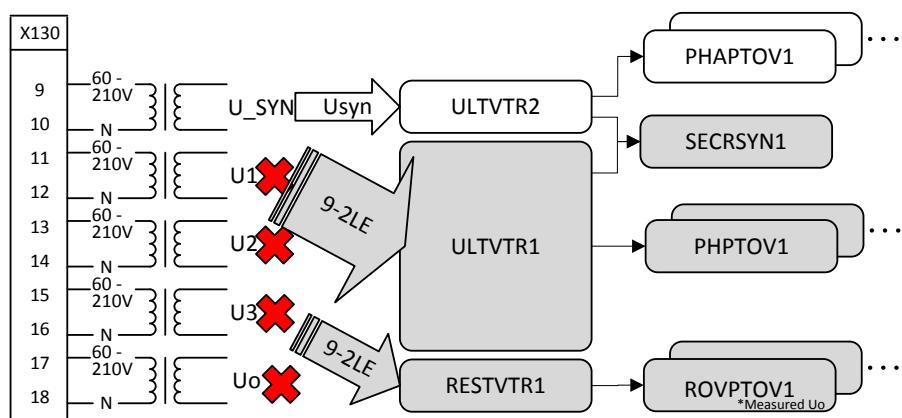
Figure 54: Both ULTVTR1 and RESTVTR1 use voltages from received IEC 61850-9-2 LE sample value
