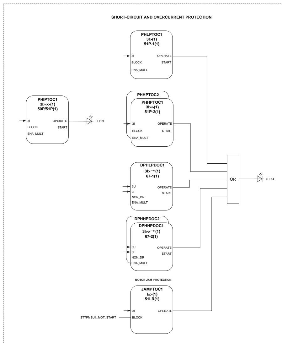
Figure 23: Overcurrent and motor jam protection
