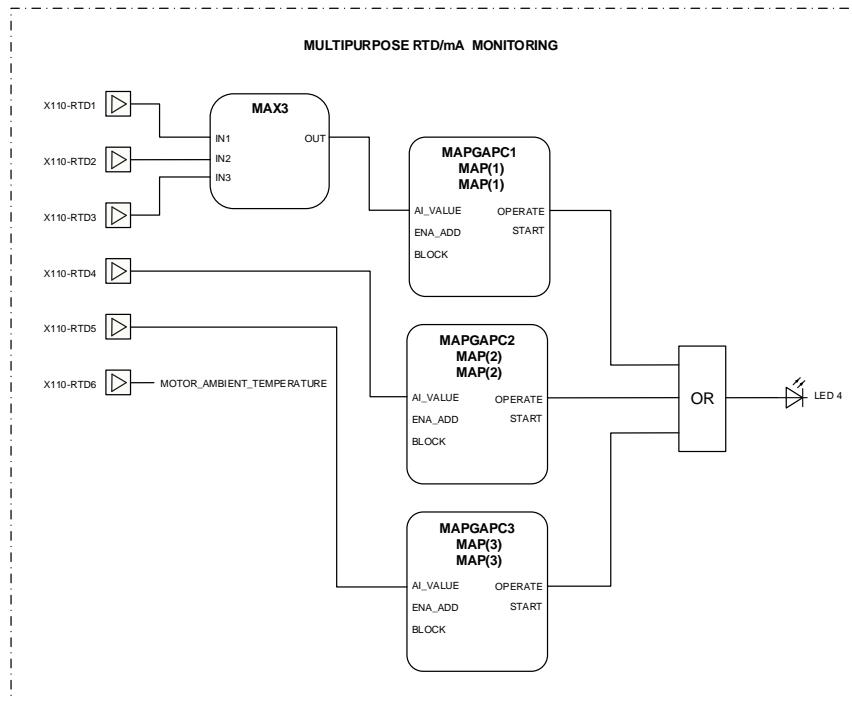
*Figure 33: Multipurpose RTD/mA monitoring*
