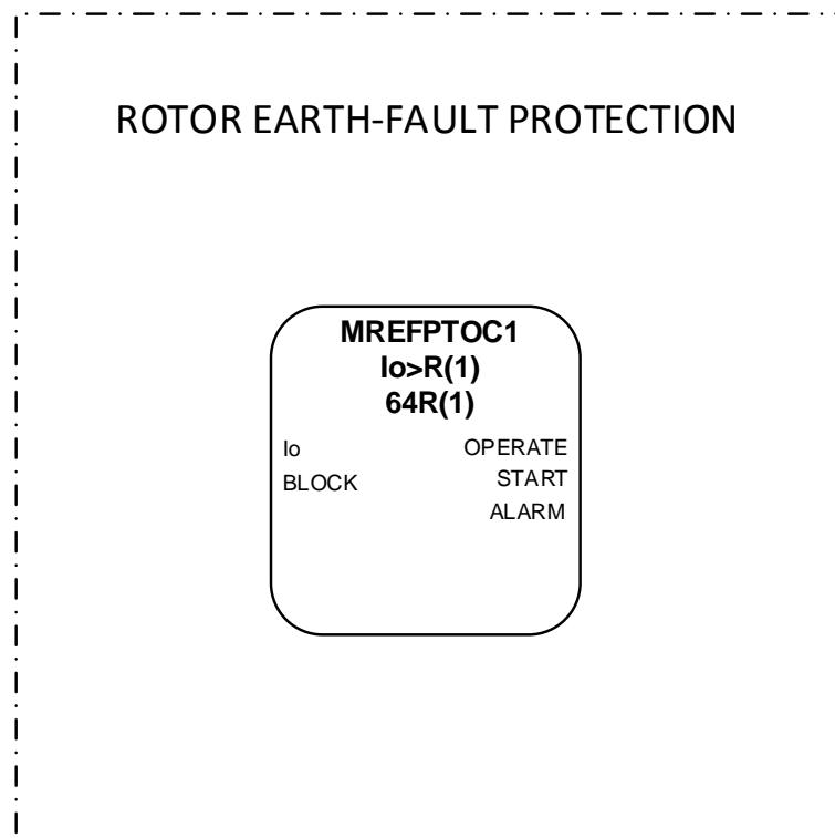
*Figure 78: Rotor earth-fault protection*
