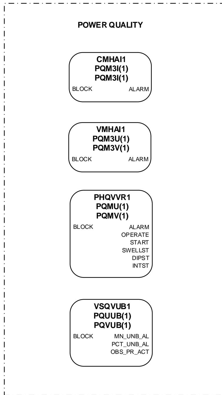
Figure 76: Power quality measurement function
