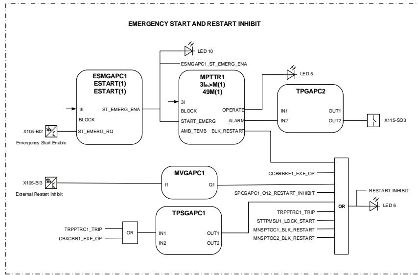
Figure 65: Emergency start and restart inhibit
