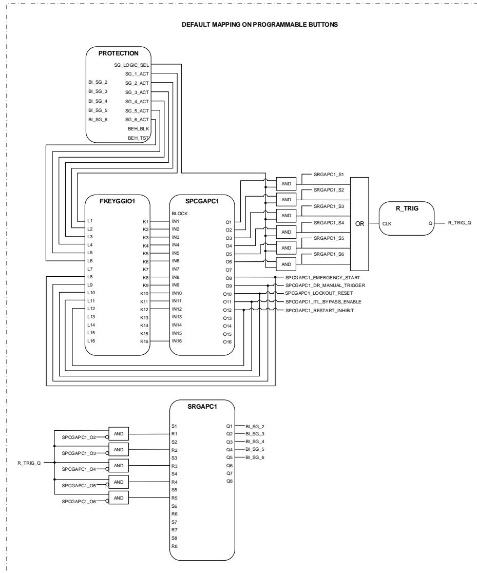
Figure 59: Default mapping on programmable buttons
