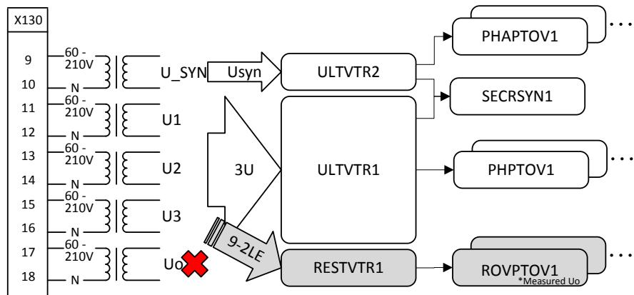
Figure 52: RESTVTR1 uses residual voltages from received IEC 61850-9-2 LE sample value
