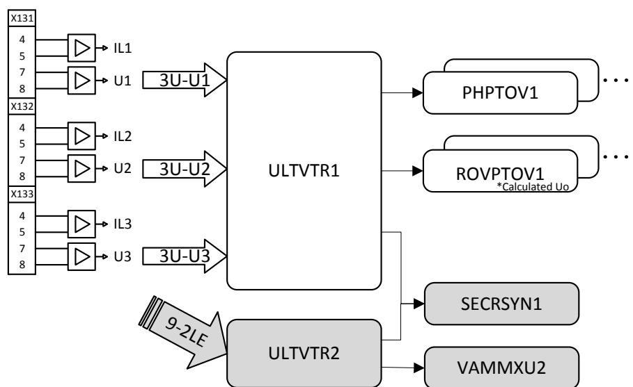
Figure 86: ULTVTR2 uses UL1 voltage from received IEC 61850-9-2 LE sample value
