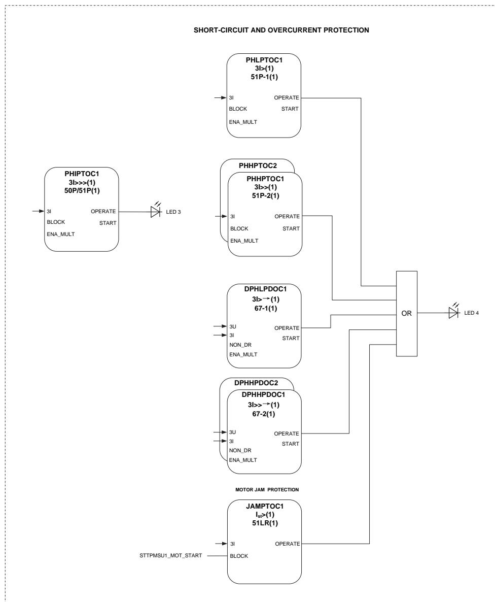
*Figure 60: Overcurrent and motor jam protection*
