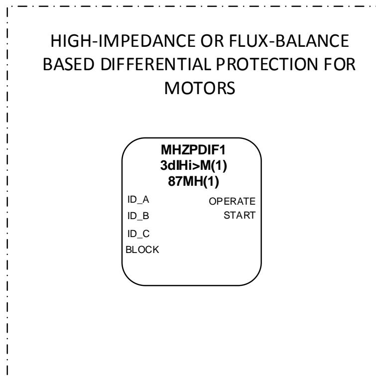
Figure 43: Flux-balance based differential protection for motors
