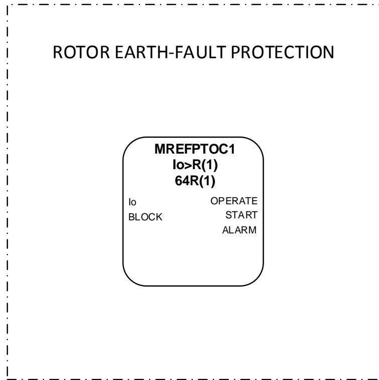
*Figure 44: Rotor earth-fault protection*
