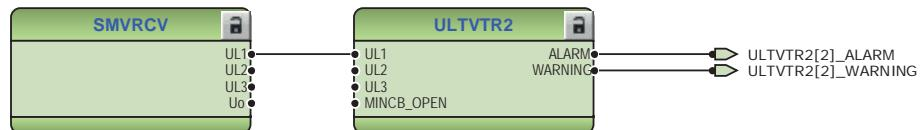
Figure 85: Connection of SMVRCV to ULTVTR2 in Application Configuration
