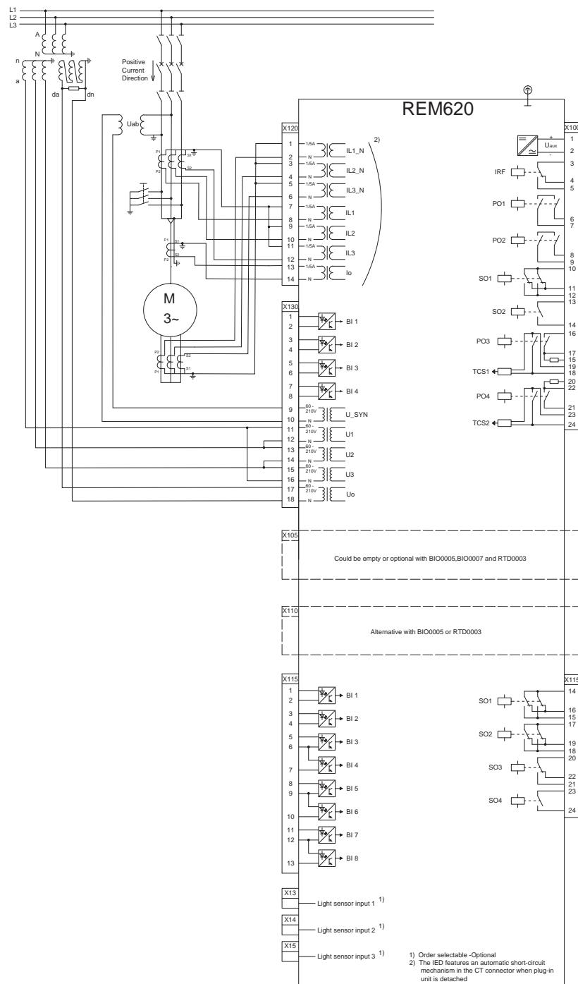
Figure 13: Connection diagram for the A configuration
