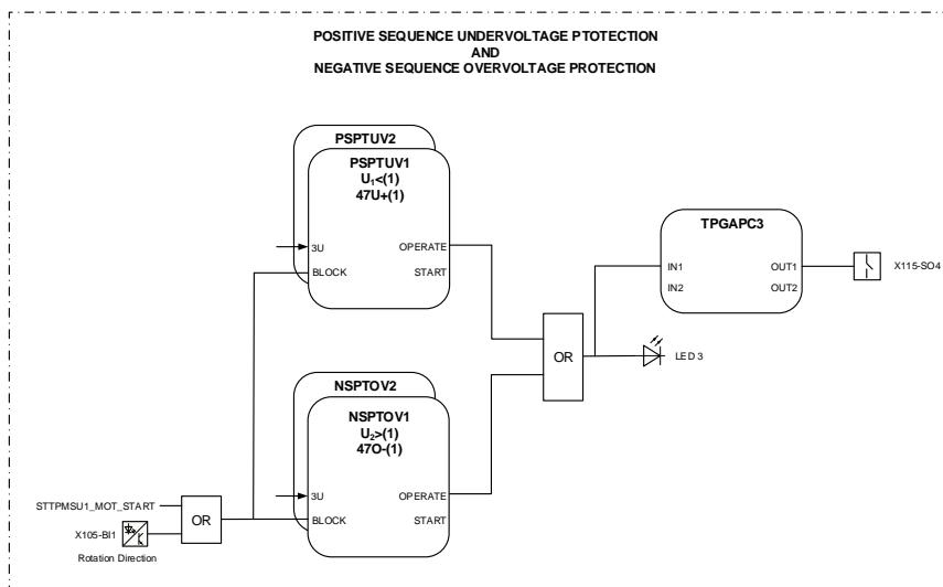
*Figure 63: Positive-sequence undervoltage and negative-sequence overvoltage protection*
