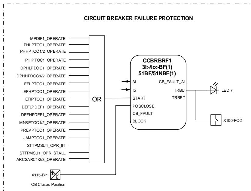
*Figure 32: Circuit breaker failure protection*
