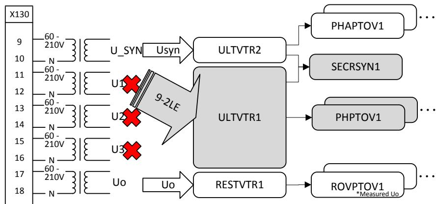
Figure 50: ULTVTR1 uses three phase voltages from received IEC 61850-9-2 LE sample value
