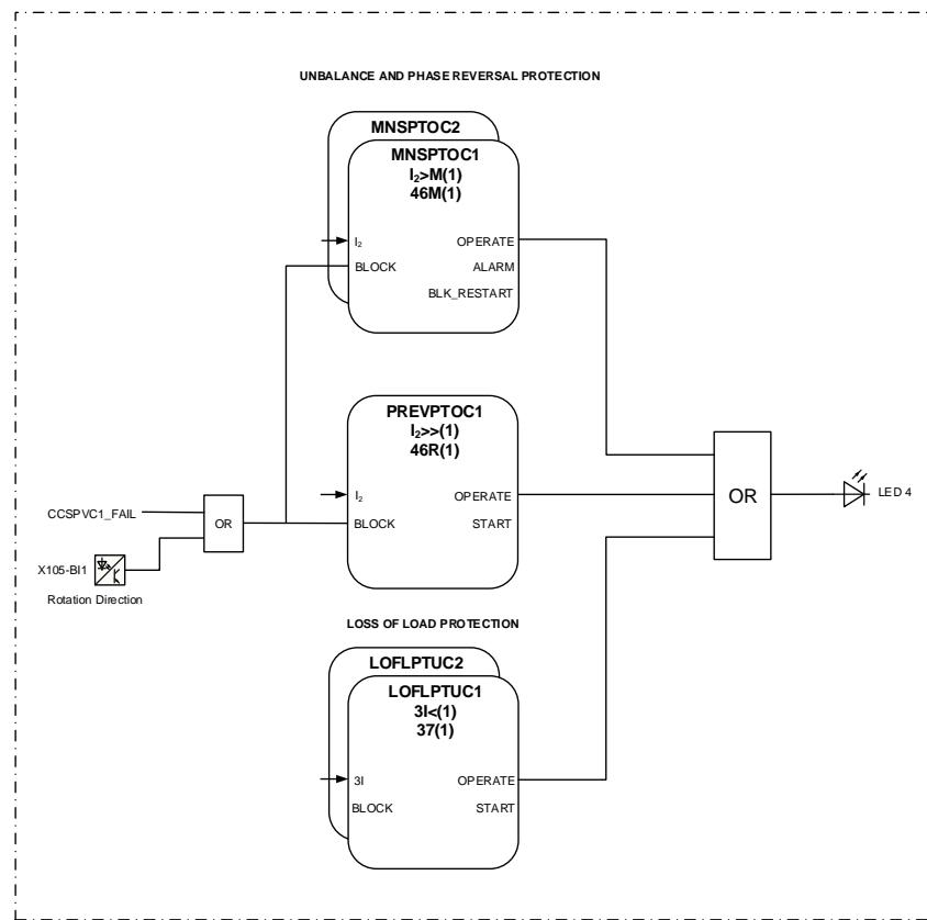
*Figure 67: Phase unbalance and loss of load protection*
