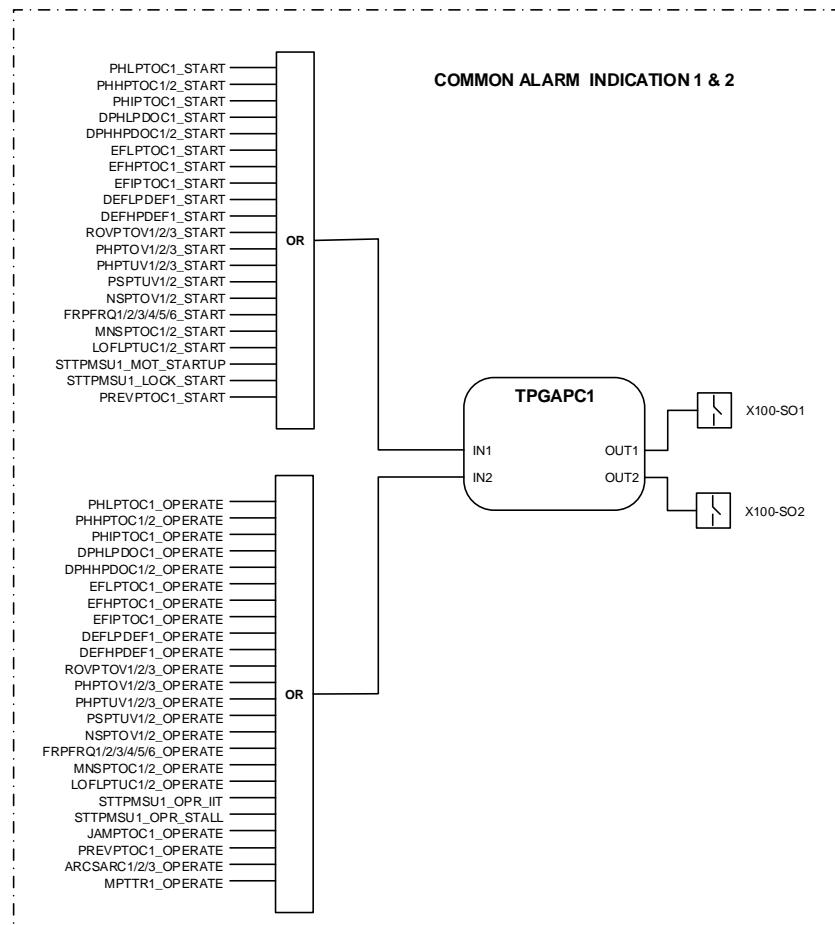
*Figure 75: Common alarm indication*
