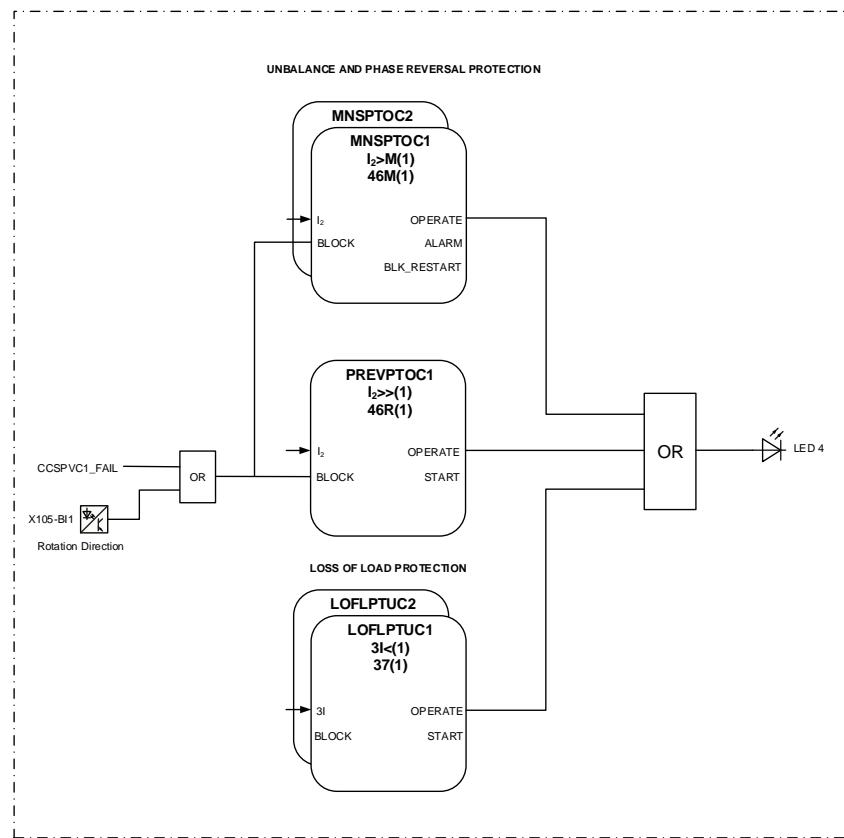
*Figure 30: Phase unbalance and loss of load protection*
