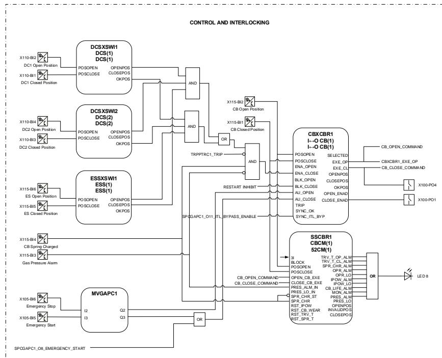
Figure 74: Circuit breaker control and interlocking
