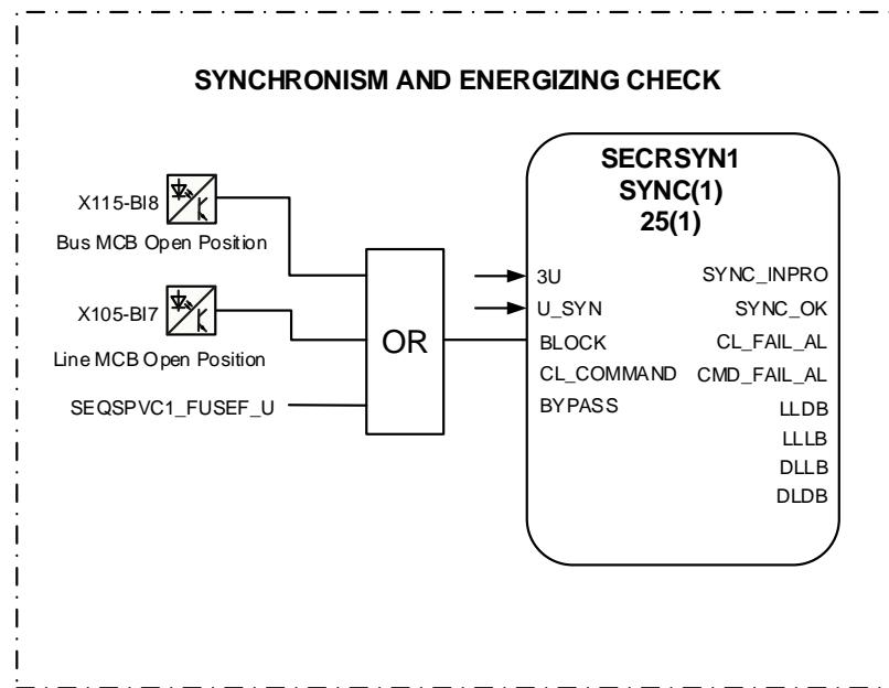
Figure 37: Synchronism and energizing check
