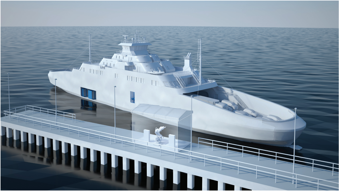
Automatic shore connection enabled by the ABB Robotic solution
