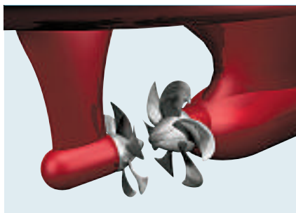
4 Contra-rotating propellers improve the vessel's hydrodynamic performance.
