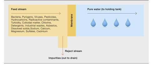
brane generates osmotic pressure. Applying an external pressure to reverse the natural flow of pure solvent is reverse osmosis. For drinking water, the pressure forces only the water molecules through the membrane, resulting in clean water on the other side. Different pressures are applied depending on which dissolved contaminants are present.
