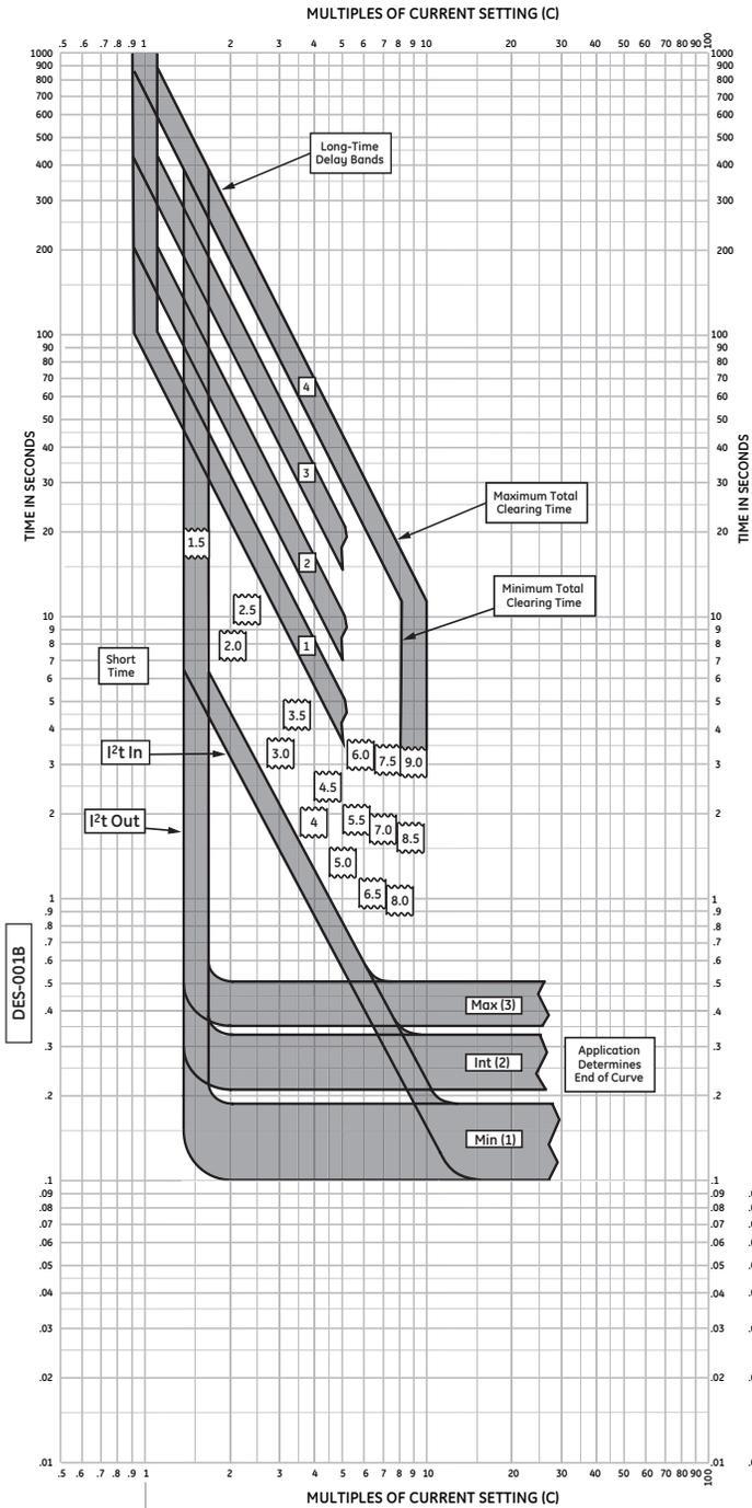
**MVT Instantaneous Pickup Settings in Multiples of Rating Plug Amps (X)**
