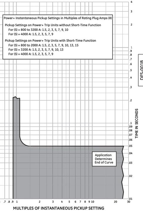
**Power+ Instantaneous Pickup Settings in Multiples of Rating Plug Amps (X)**
