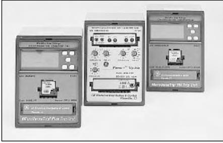
There are three trip unit systems available for WavePro™ Low Voltage Power Circuit Breakers — Power+, and enhanced MicroVersaTrip Plus and MicroVersaTrip PM. All three systems consist of the trip unit, the trip actuator, current sensors and rating plugs. The term “trip unit systems” applies to the combination of these four components, which form the circuit breaker solid-state tripping system.
