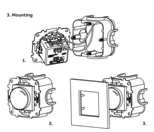
Turn the device in the correct installation position. The marks on the back side of the device, orients the correct top position.
