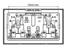
Distance between fixing screws for 2 gang frames
