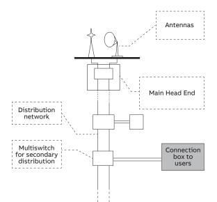
a) SMATV star connection diagram 8151.3 or N2251.3 Final 00 Derivation losses
