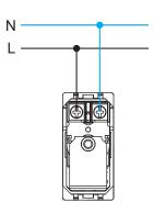
Note: the buzzer is set for 230Vac operation. For other voltages, the tone must be adjusted by means of the screw regulator on the back.
