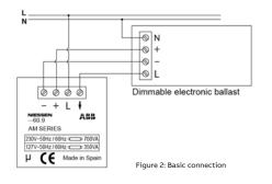
The maximum charge to be connected to the control terminals +/should not exceed 50 mA.
