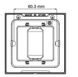
Distance between fixing screws for 1 gang frames
