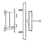
**2.** There are two options of mounting the cover plates: a) cut the clamps that are facing the small holes.
