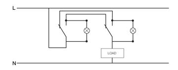
The two warning lights switch on and off respectively
