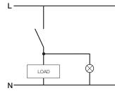
Warning light placed in parallel to the load, of which indicates the ON/OFF state (it is on when the switch is ON).
