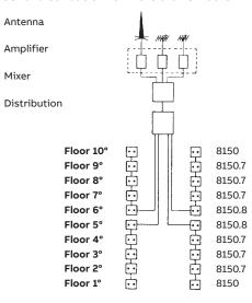
Example: 10 floors. The floors are divided in 2 groups of 5 floors each. The outlets are distributed according to the criteria shown in the MATV connection diagram for serial distribution up to 9 floors. The diagram above can be used in buildings up to 18 floors. For buildings with more than 18 floors and up to 27 floors, 3 groups have to be created and so on.
