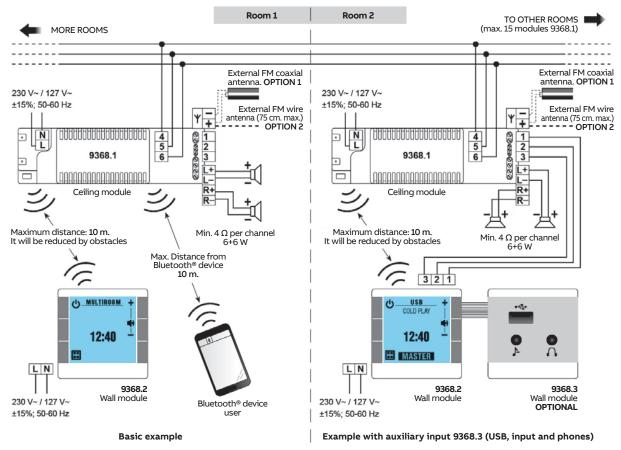
**NOTE**: Because these devices are radio frequency and to avoid interference, you should not install modules of the same reference or any other RF equipment that could interfere less than 1 m. away. It should be noted that any obstacle between the devices, can significantly reduce the distance range between them.
