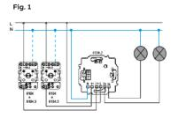
8130.2 with auxiliary buttons (8144.2, 8104.5) and two lamps.
