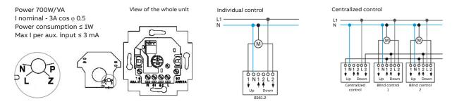
The IR button 8439.XX and the programmer 8165.3 can control a group of blind motors by operating the auxiliary inputs ("1" and "2") of the blind control device. Using a two-pole switch for blinds, the group of blinds can be moved manually or the sensor can be activated for periods of absence. The recessed device 8161.2 is used to control:
