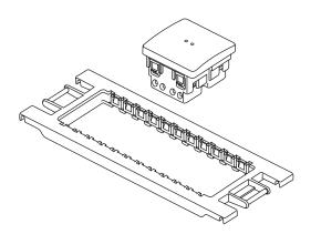
**2.** Both in the surface solution and in the flush solution, there are metal mounting plates where the mechanisms are inserted.
