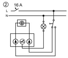
Operation in a two-way circuit
