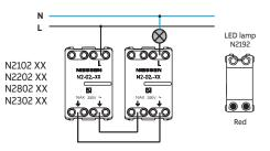
2-way switch - Intermidiate switch - 2-way switch
