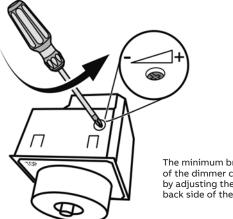
The minimum brightness of the dimmer can be set by adjusting the on the back side of the device.
