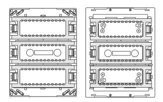
3. The mechanisms are inserted in the mounting plate by pressure.
