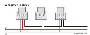
Terminals 3 and 4 are connected via the internal contact to the telephone (closed with the receiver hung up). Lifting the receiver causes interruption of the downstream line (L1), guaranteeing secrecy of the conversation.
