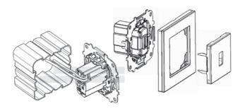
3.3.- Fig. 5. -Installation of USB charger with two outlets 8185.3
