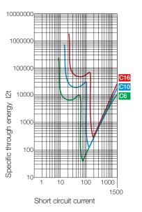
Current-time tripping diagrams for circuit-breakers of the Chiara range
