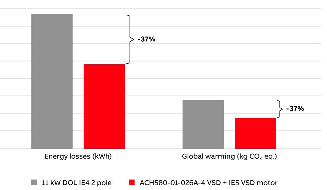
Use stage energy losses and contribution to global warming of ACH580-01-026A-4 VSD + IE5 VSD motor system and an equivalent DOL motor.
