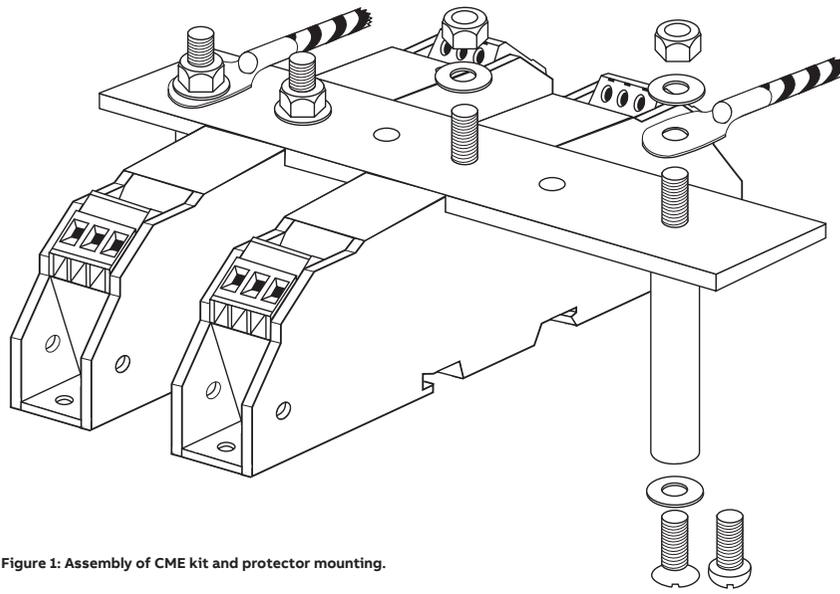
Figure 1: Assembly of CME kit and protector mounting.
