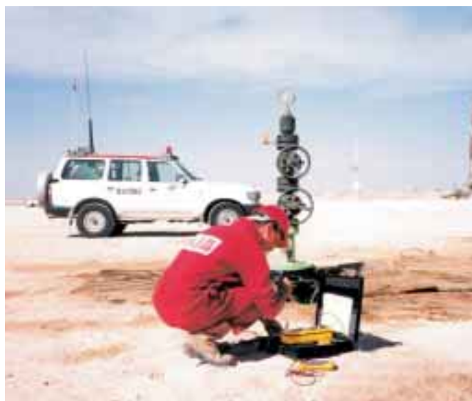
An ABB engineer tests and verifies borehole instrumentation strings in the Yibal oil and gas field – courtesy of PDO and the Oman Ministry of Oil and Gas.
