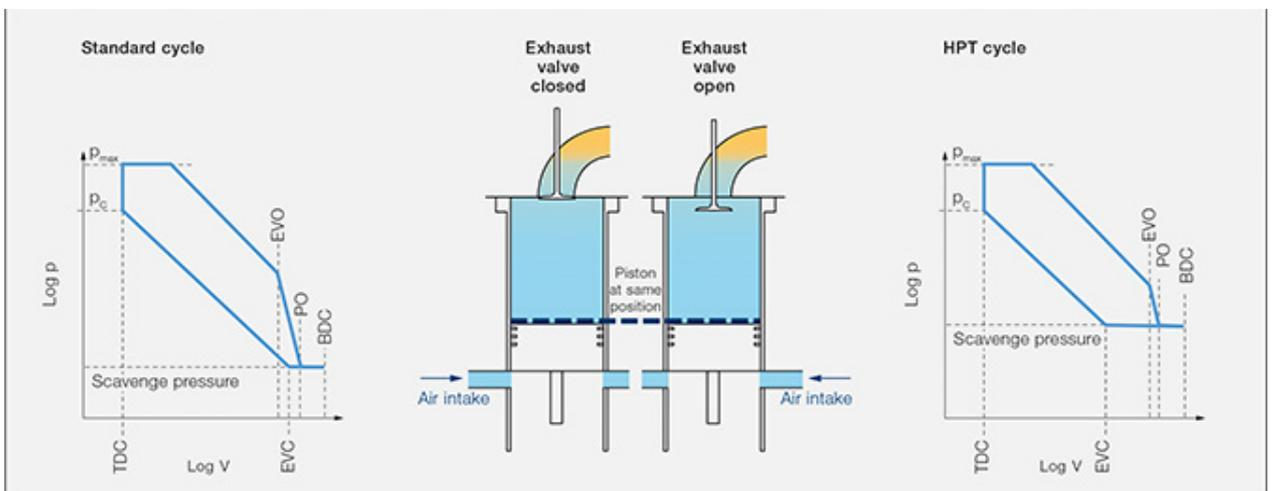
Fig. 2: Standard versus HPT cycle
