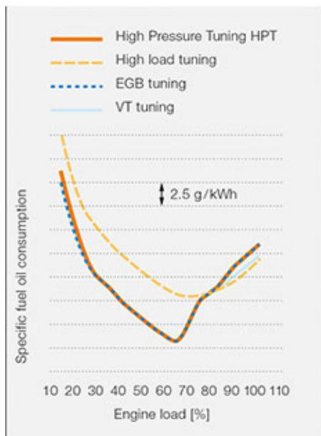
Fig. 4: Specific fuel oil consumption tuning curve
