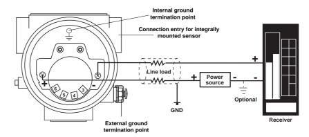
**NOTE**: Use terminals 3 and 6 for external CJC of thermocouple (if any by Pt 100)
