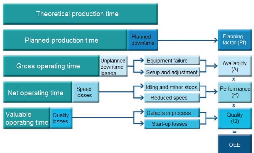
Figure 2. OEE model, in the context of plant electrical equipment.
