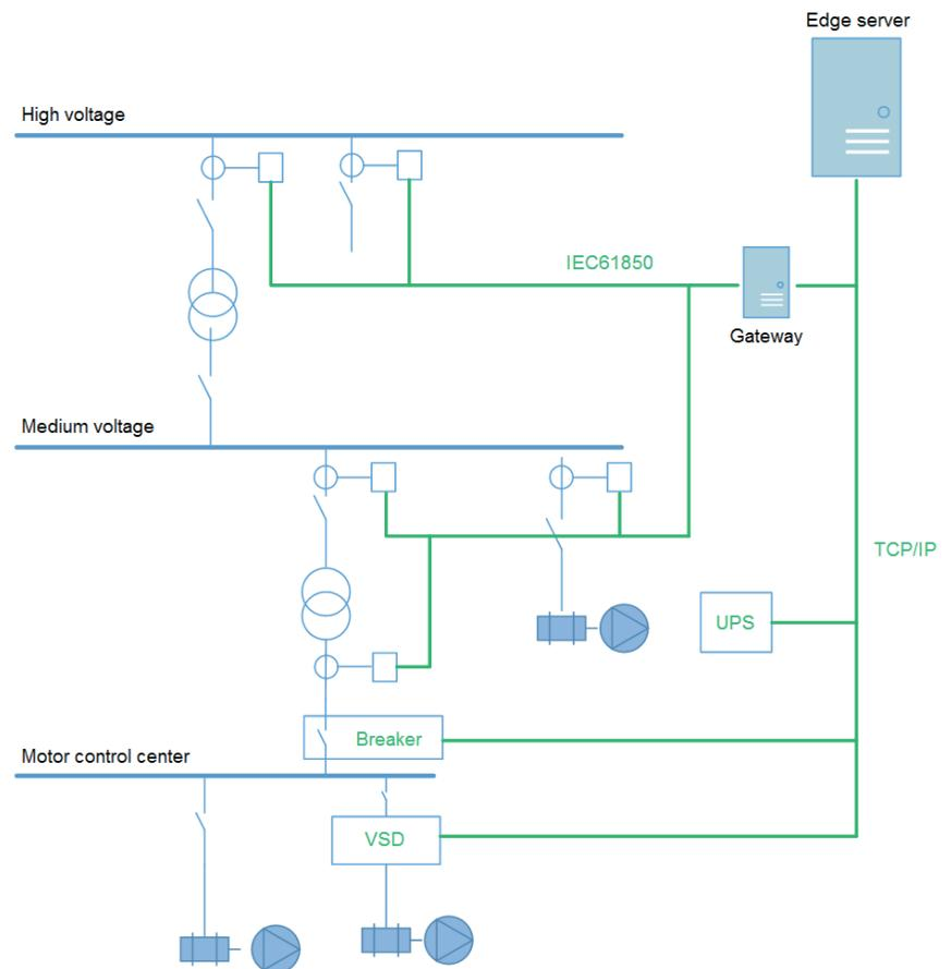
**Figure 3.** Metsä Fibre's condition monitoring architecture for its electrical system.
