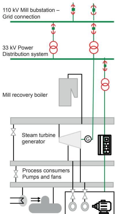
**Figure 1.** A typical pulp mill power system.
