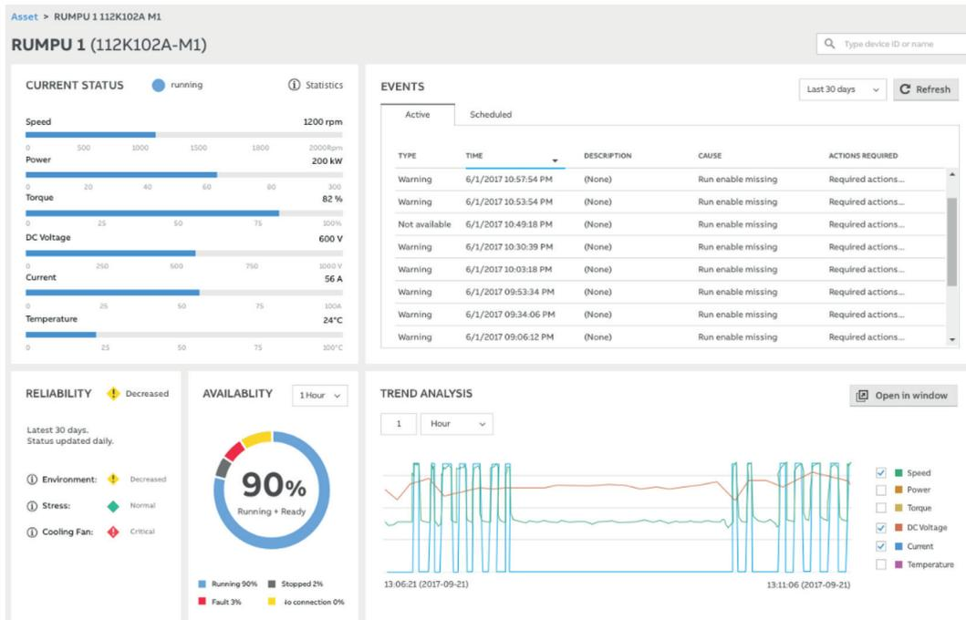
Figure 5. Example of equipment detail page in the monitoring application.
