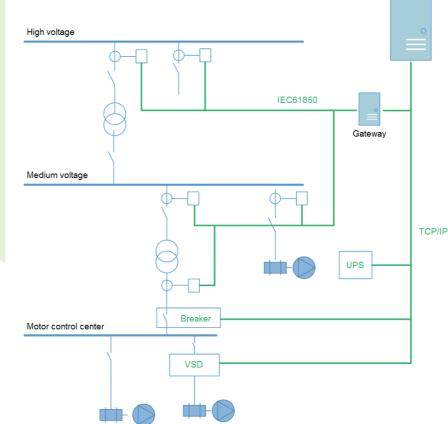
Figure 3. Metsä Fibre's condition monitoring architecture for its electrical system.
