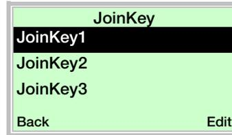
The four numbers of the JoinKey are again separated as 8 single hexadecimal characters 0 ... 9 + A ... F. The hexadecimal characters are set individually, one by one by using the and button to select a hexadecimal character. As the JoinKey can not read back for security reasons the selected character after entering the sub menu is "8" always.
