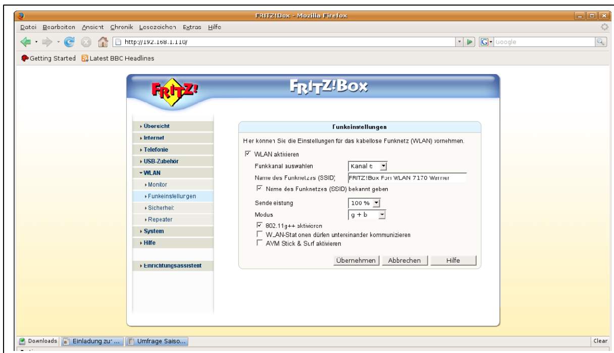
Figure 5: basic settings for the Wi-Fi base station on the Fritz!Box 7170
