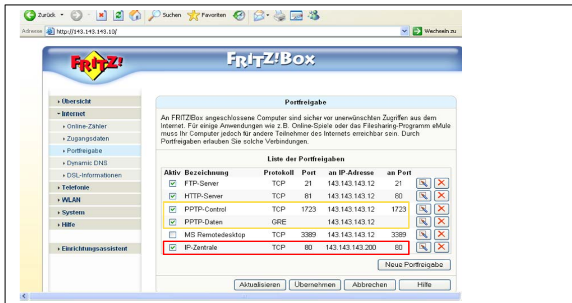
Figure 5: port forwarding configuration on the Fritz!Box 7170
