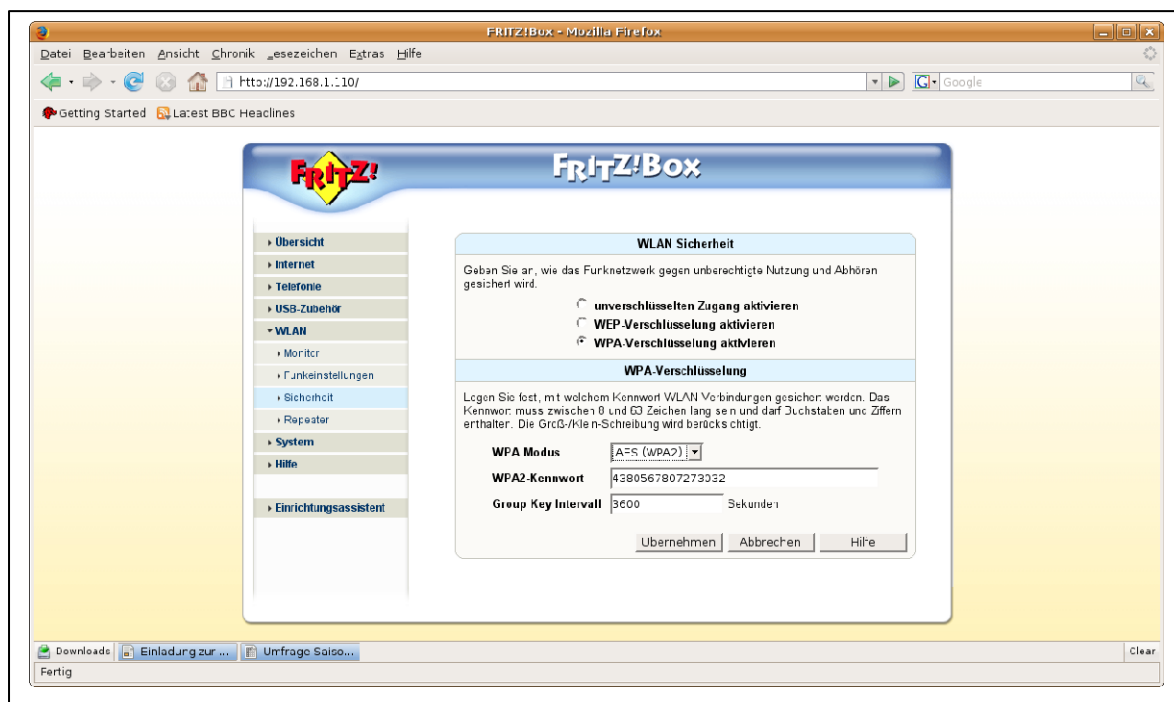
Figure 6: configuring security settings for the Wi-Fi base station on the Fritz!Box 7170
