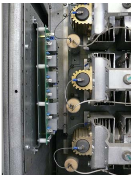
PIN48/51 Mounting Kit standard in Power stack
