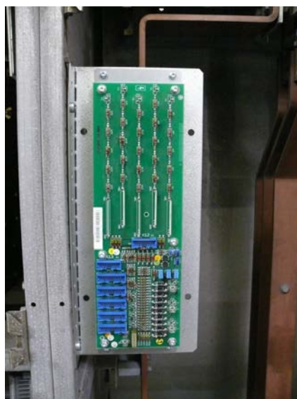
PIN48/51 Mounting Kit standard in front of power stack
