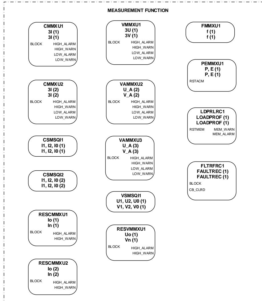
Figure 42: Measurement function
