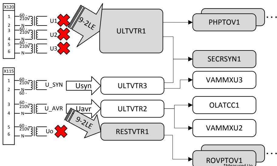
*Figure 50:* Both ULTVTR1 and RESTVTR1 use voltages from received IEC 61850-9-2 LE sample value
