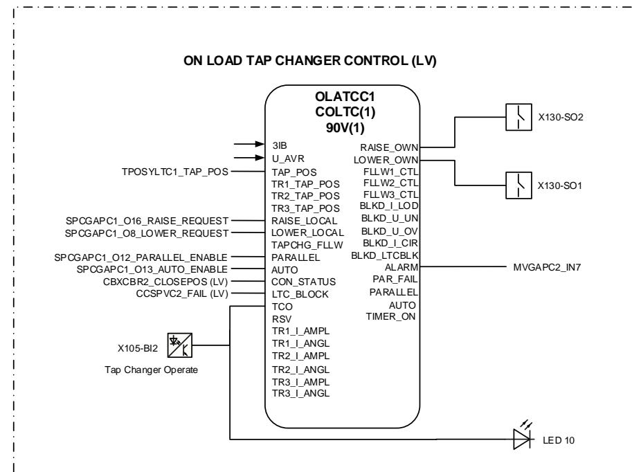
*Figure 40: On-load tap changer control*
