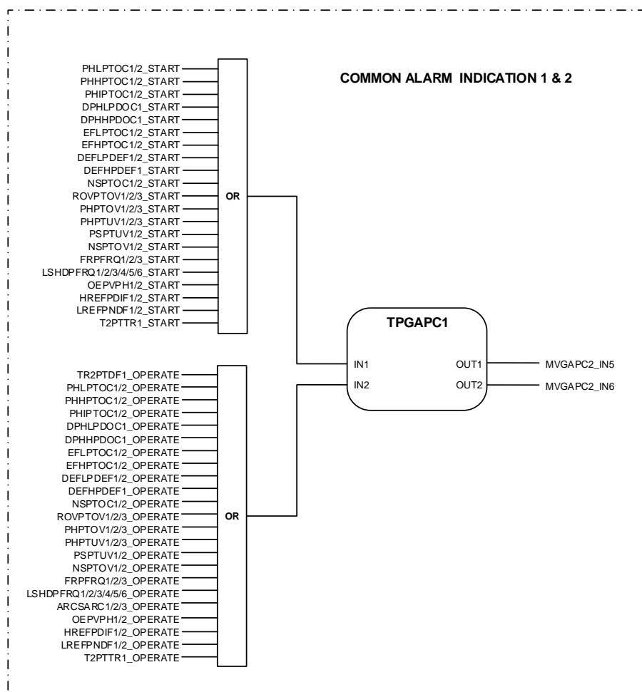
*Figure 38: Common alarm indication*
