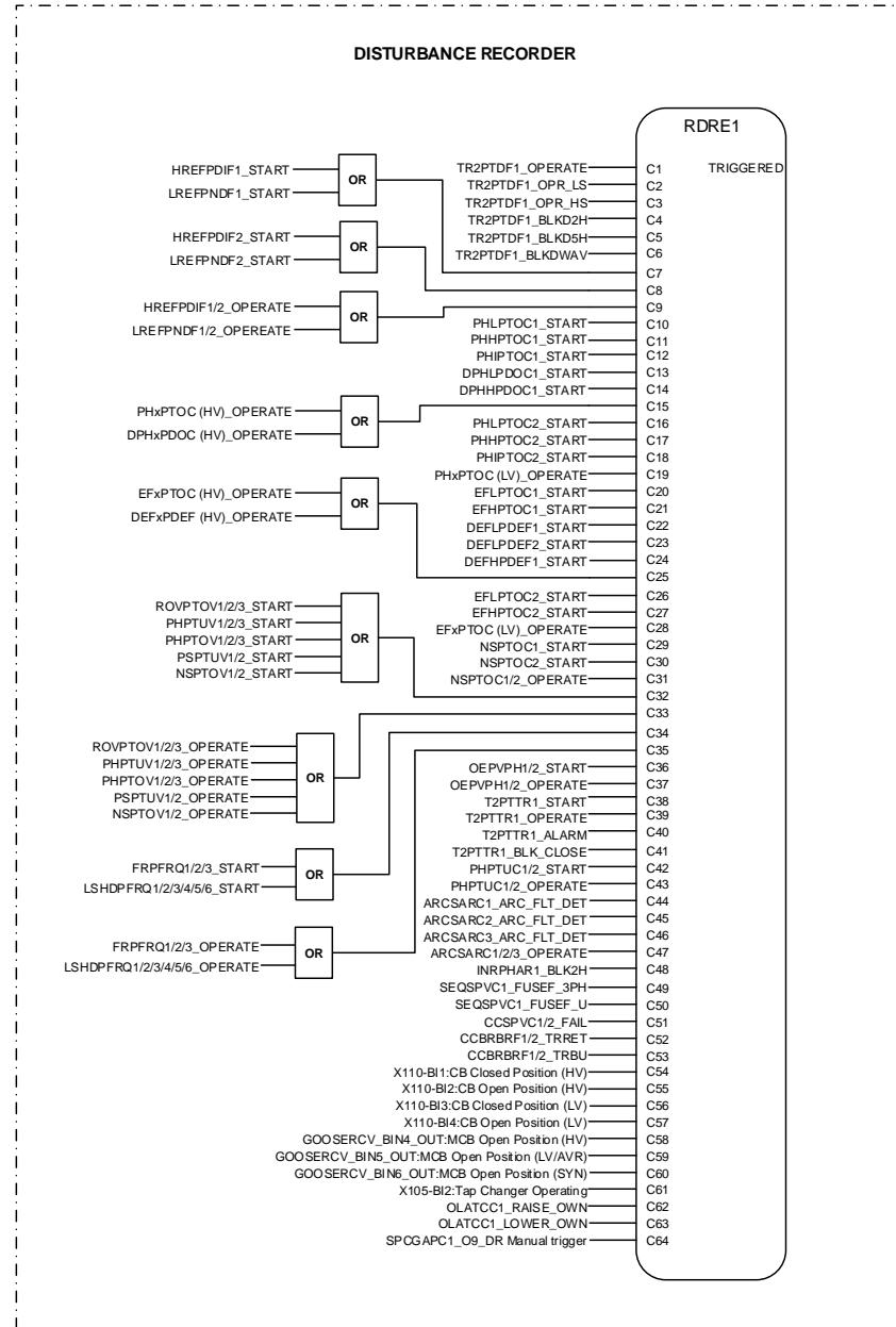
Figure 32: Disturbance recorder
