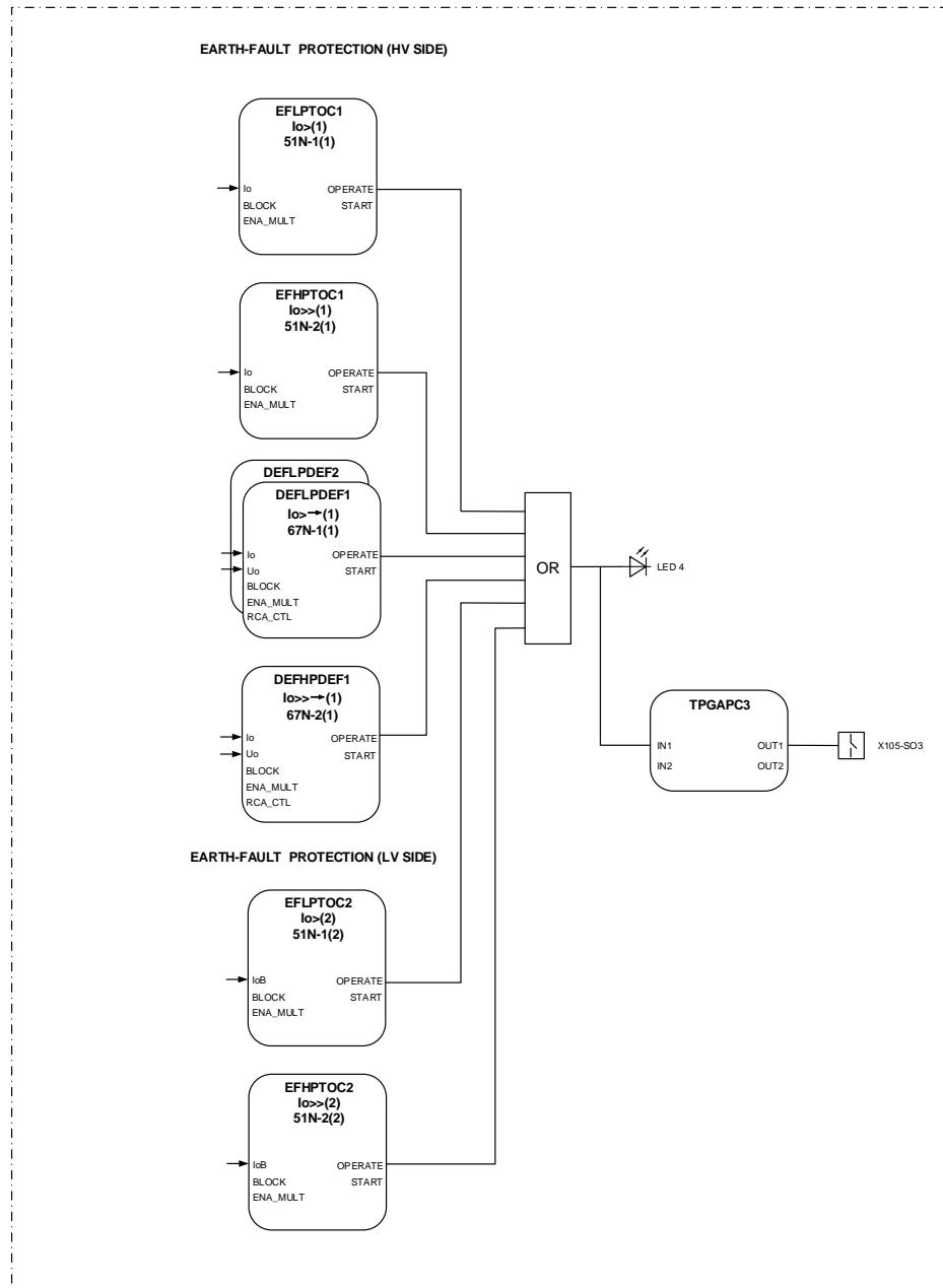
Figure 22: Earth-fault protection
