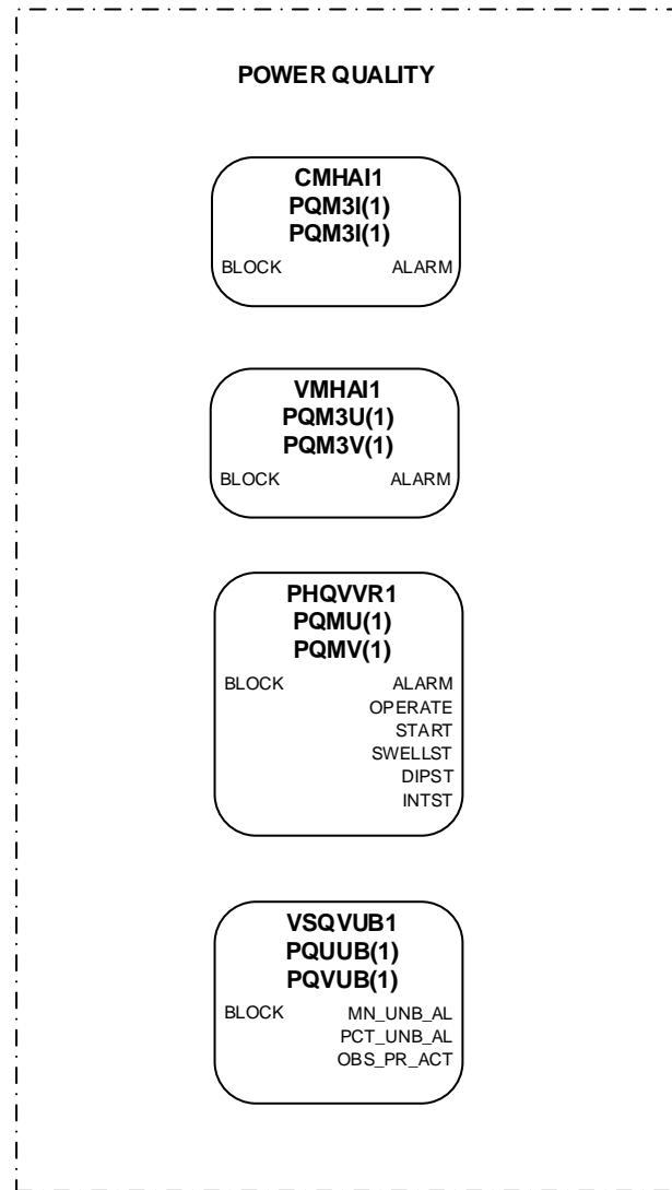
*Figure 41: Power quality measurement function*
