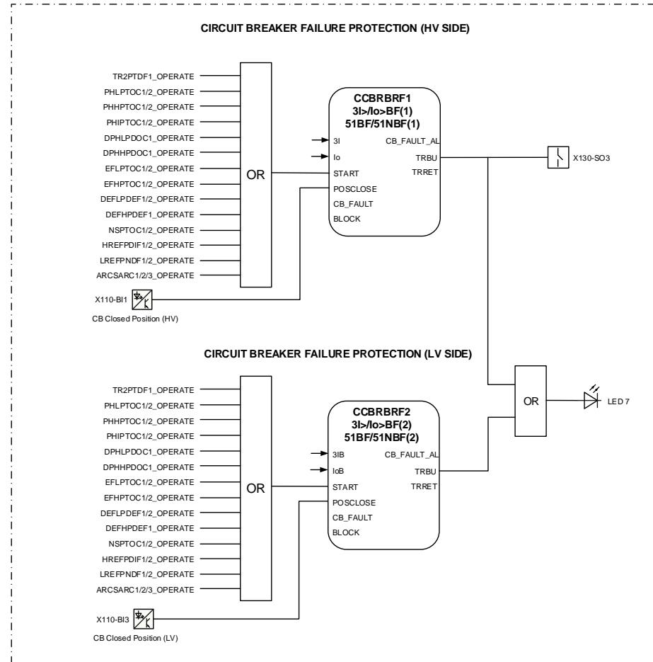
*Figure 30: Circuit breaker failure protection*
