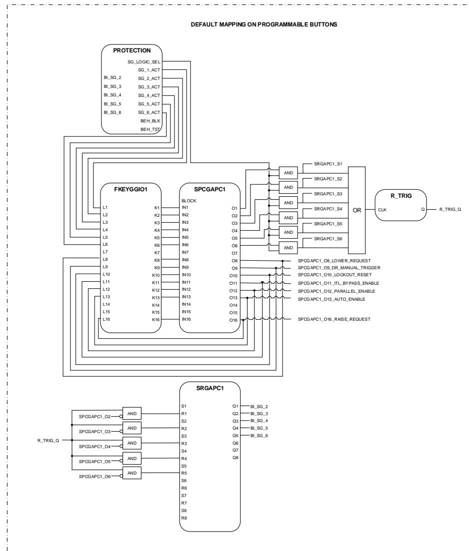
Figure 19: Default mapping on programmable buttons
