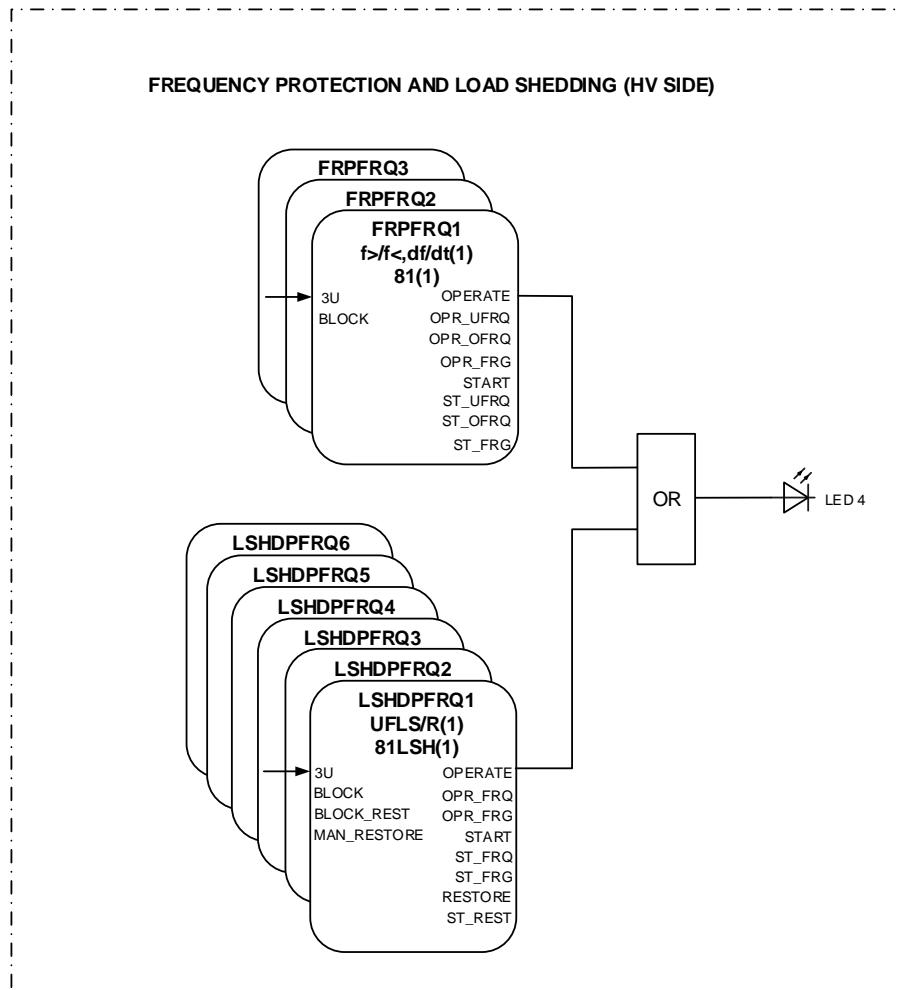
Figure 29: Frequency and load shedding protection
