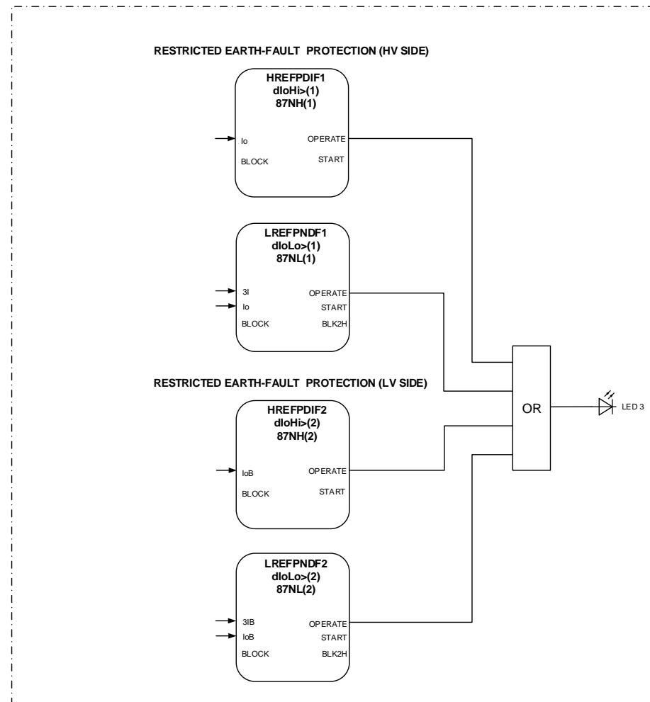
*Figure 23: Restricted earth-fault protection*
