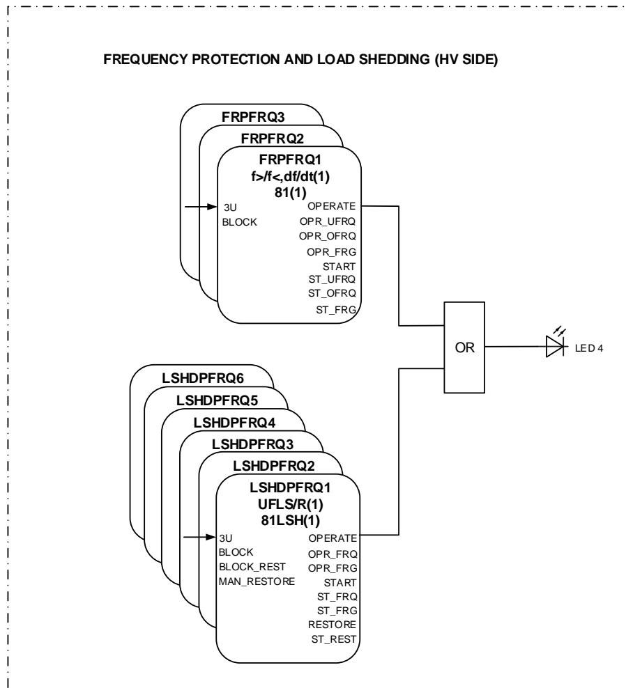
Figure 29: Frequency and load shedding protection
