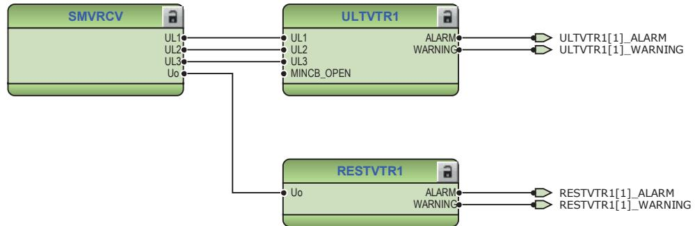
*Figure 49:* Connection of SMVRCV to both ULTVTR1 and RESTVTR1 in Application Configuration
