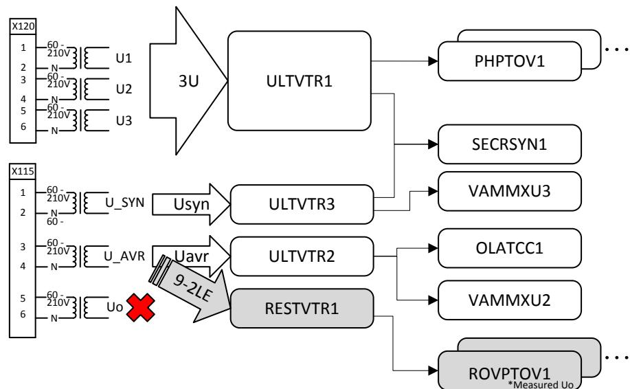
Figure 48: RESTVTR1 uses residual voltages from received IEC 61850-9-2 LE sample value
