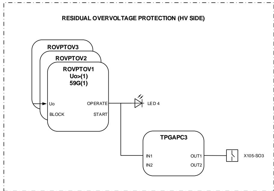
*Figure 27: Residual overvoltage protection*
