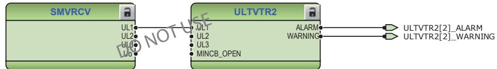
Figure 51: Connection of SMVRCV to ULTVTR2 is not supported
