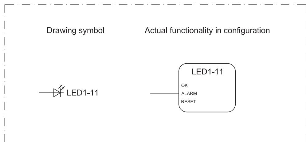
*Figure 12: Drawing symbol used in the manual and the default connection of the LED function blocks in the configurations*
