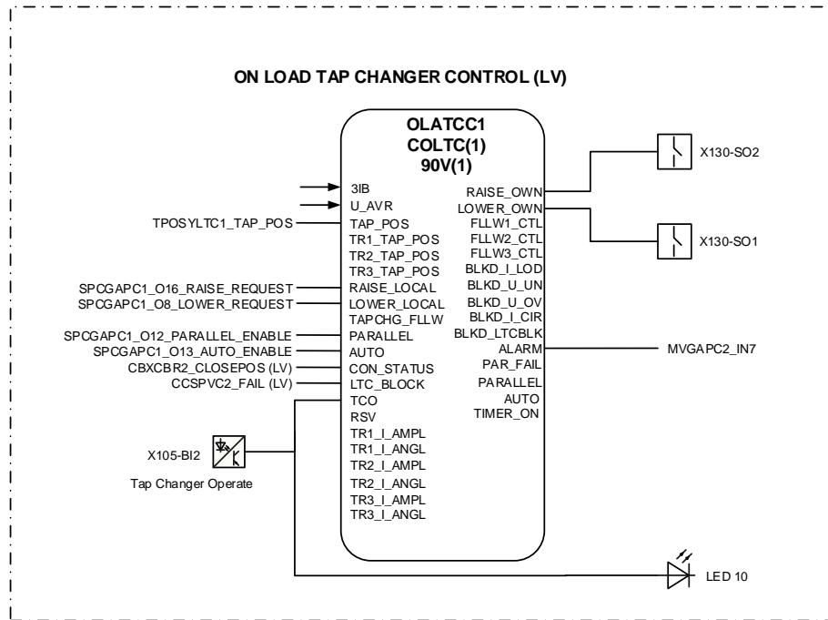
*Figure 43: On load tap changer control*
