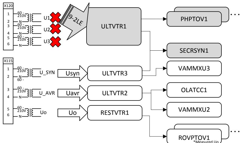
Figure 46: ULTVTR1 uses three phase voltages from received IEC 61850-9-2 LE sample value
