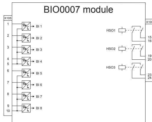
Figure 15: Optional BIO0007 module for fast outputs (slot X105)
