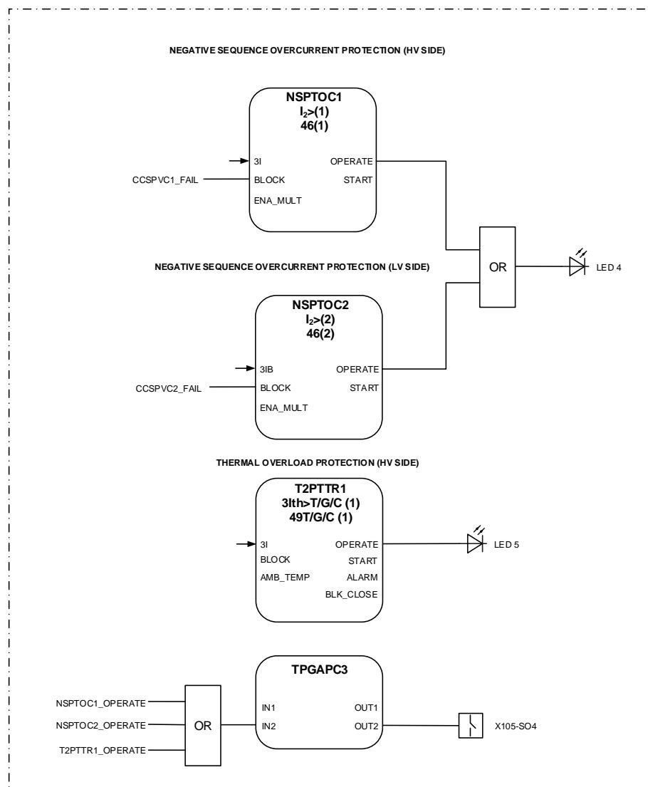
Figure 24: Negative sequence current protection and thermal overload protection
