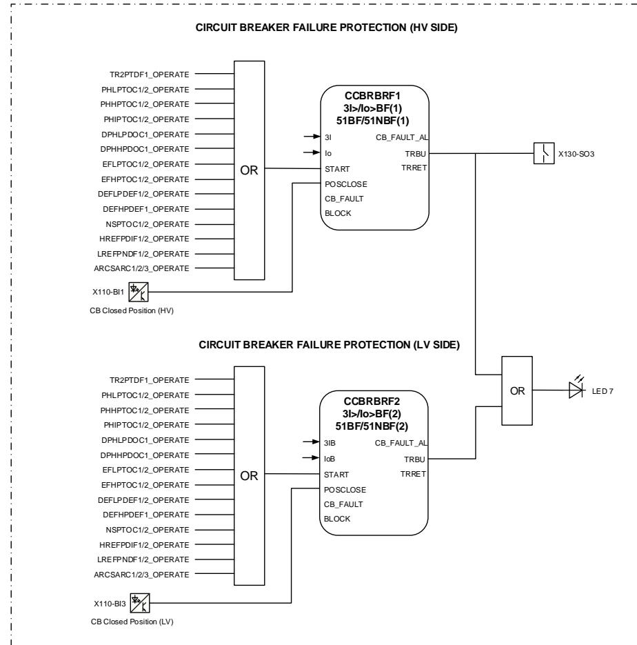
*Figure 30: Circuit breaker failure protection*
