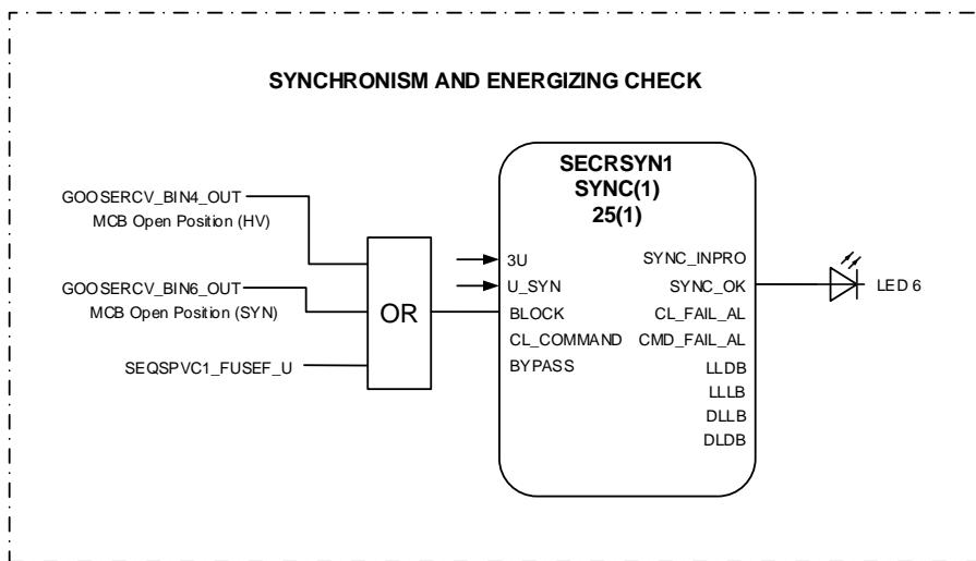
*Figure 34: Synchronism and energizing check*
