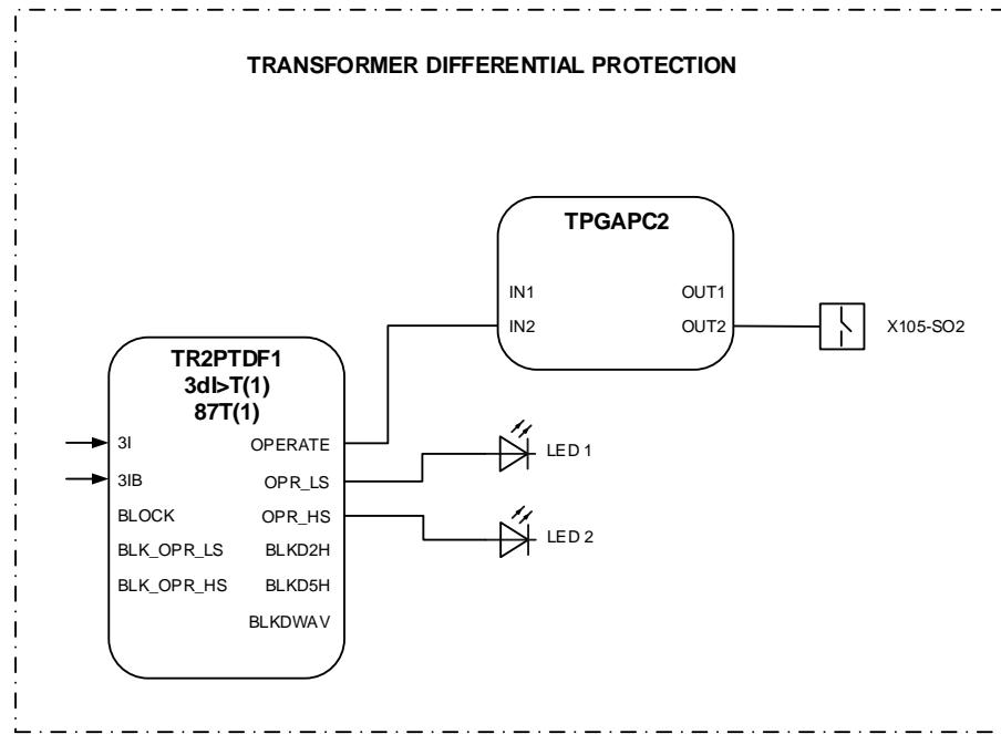
*Figure 20: Transformer differential protection*
