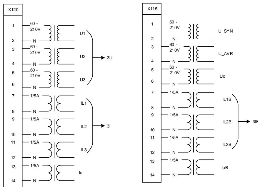
Figure 18: Physical analog channels in default configuration A
