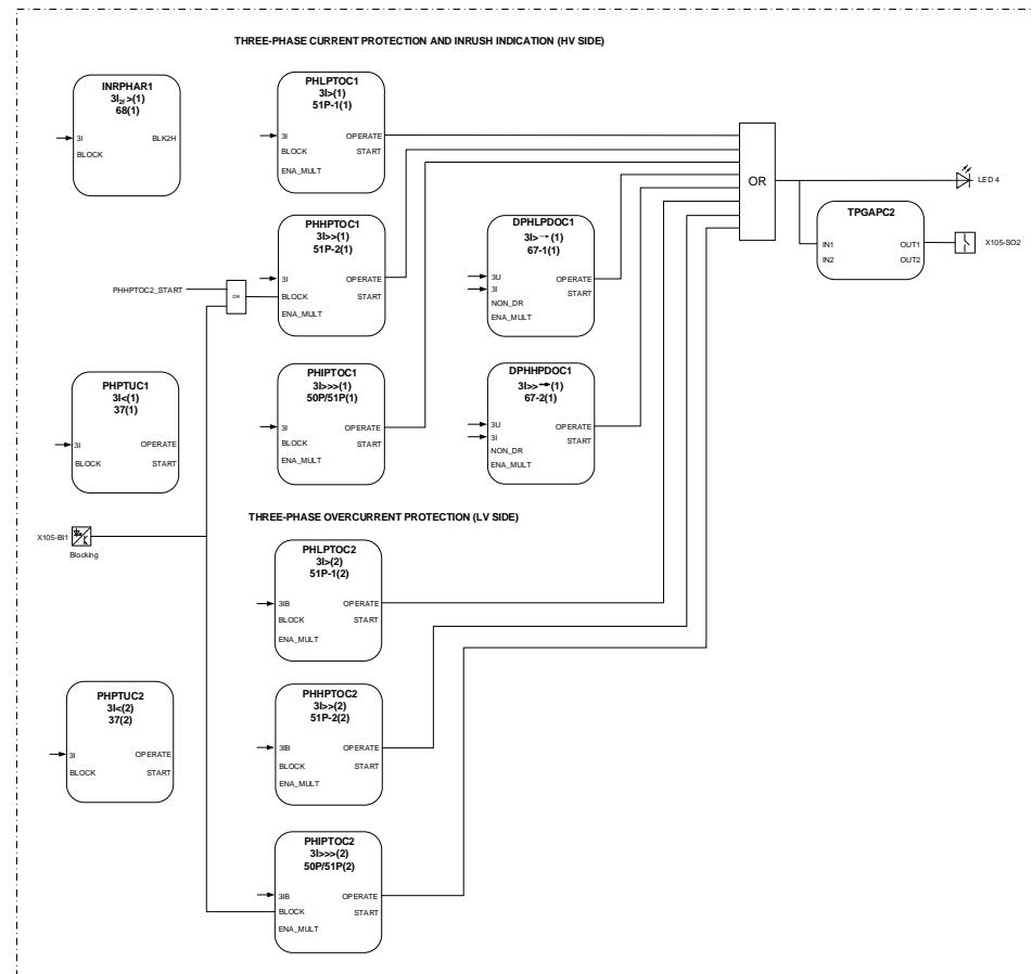
*Figure 21: Three-phase current protection and inrush indication*
