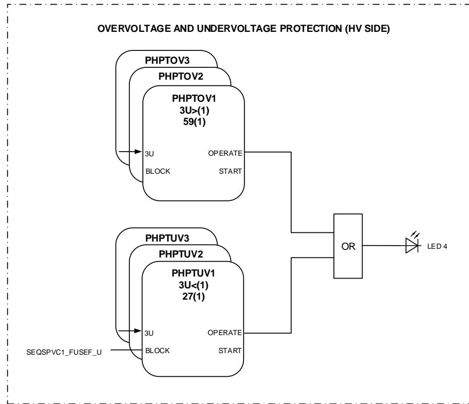
*Figure 25: Overvoltage and undervoltage protection*
