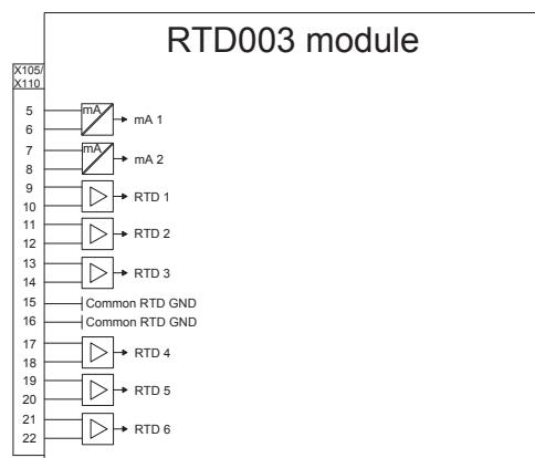
Figure 16: Optional RTD003 module (slot X105)
