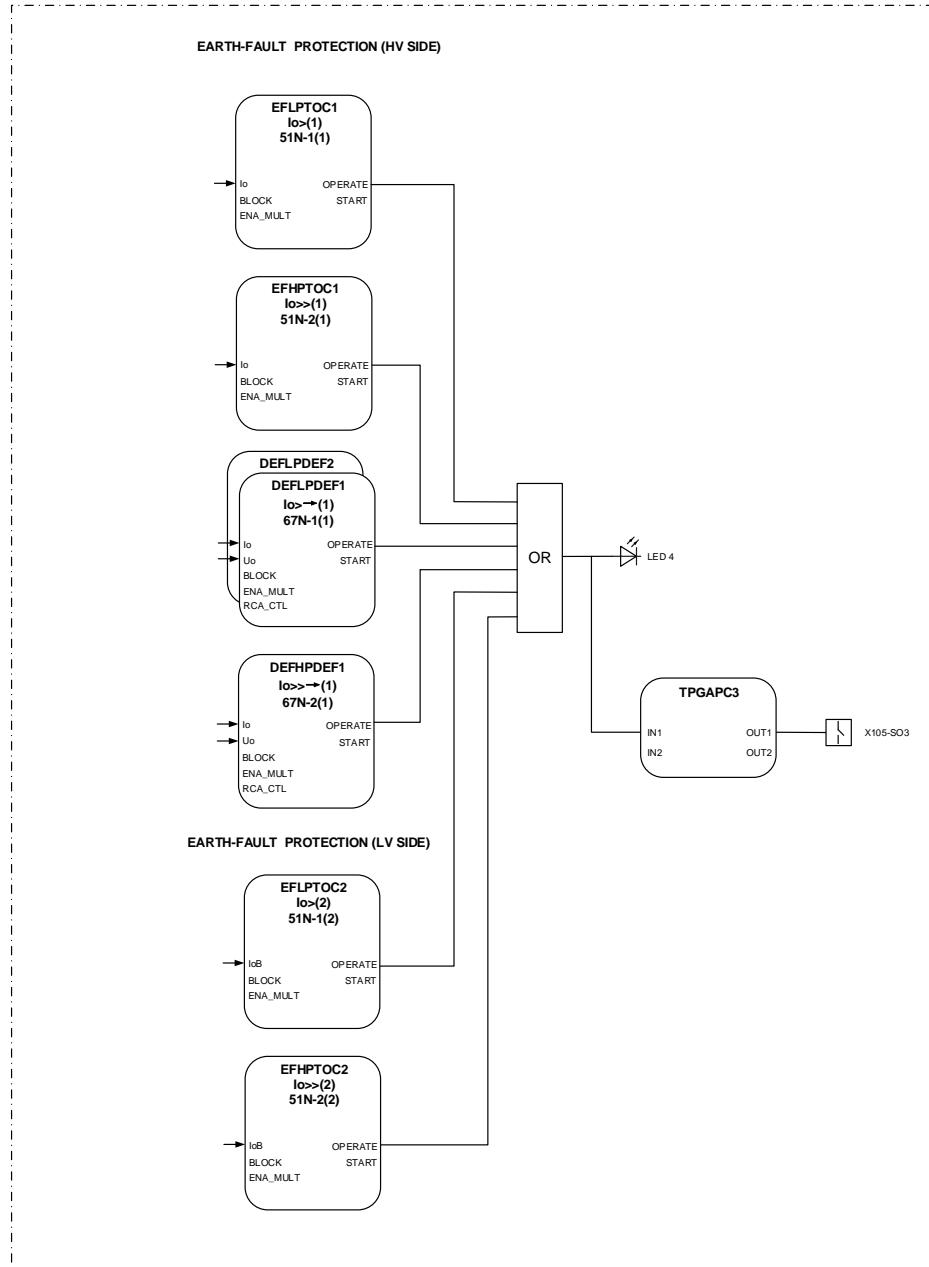
Figure 22: Earth-fault protection
