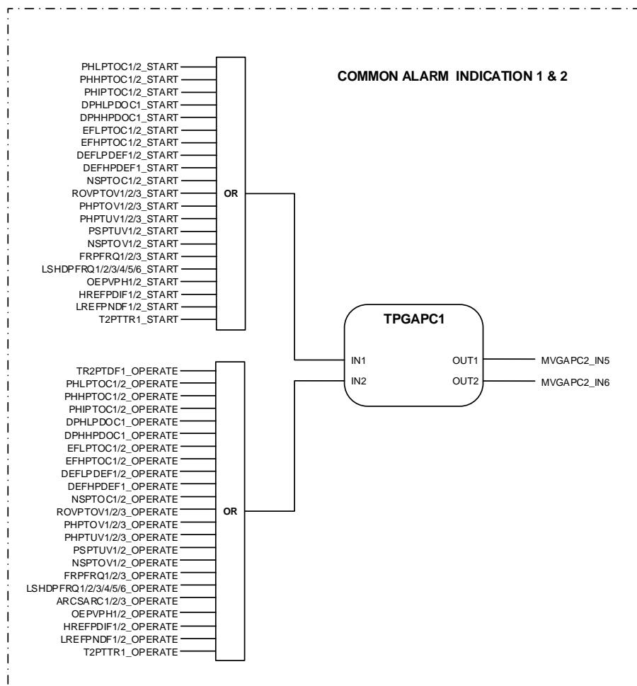
*Figure 38: Common alarm indication*
