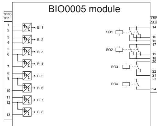
Figure 14: Optional BIO0005 module (slot X105)
