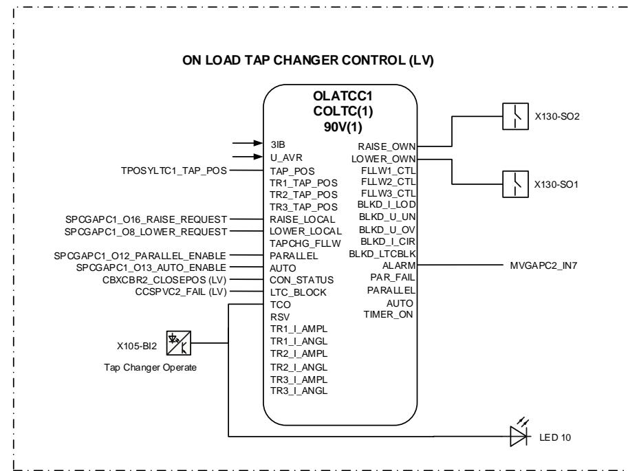
*Figure 40:* On-load tap changer control
