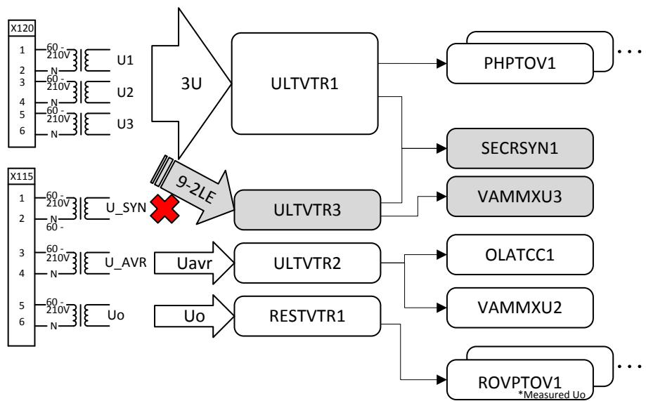
*Figure 53: ULTVTR3 uses UL 1 voltage from received IEC 61850-9-2 LE sample value*
