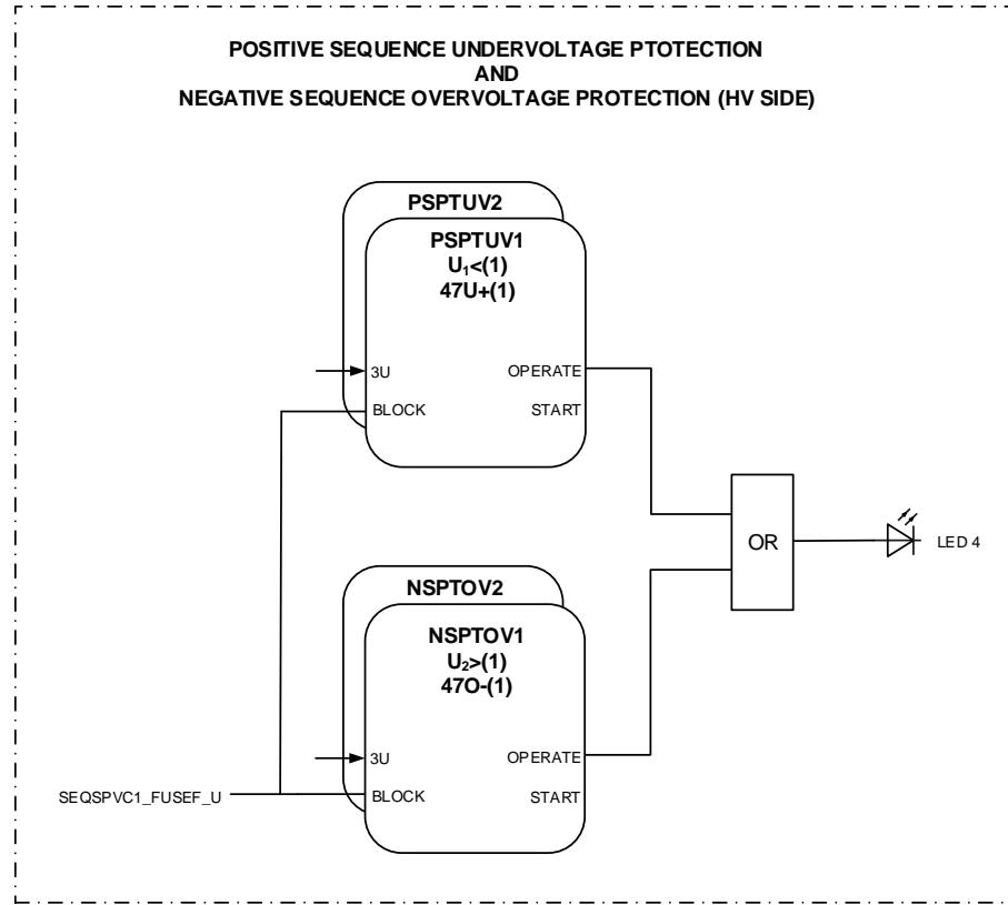
*Figure 26: Positive-sequence undervoltage and negative-sequence overvoltage protection*
