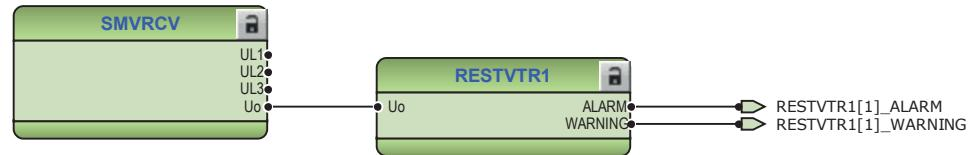
Figure 47: Connection of SMVRCV to RESTVTR1 in Application Configuration
