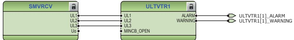
Figure 45: Connection of SMVRCV to ULTVTR1 in Application Configuration
