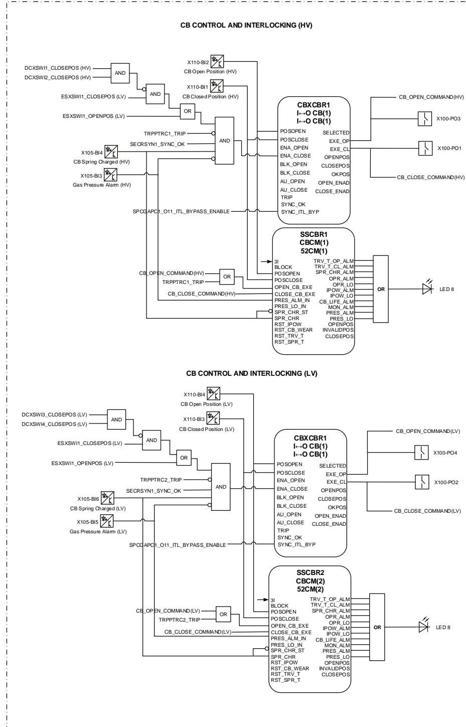
Figure 36: Circuit breaker control and interlocking
