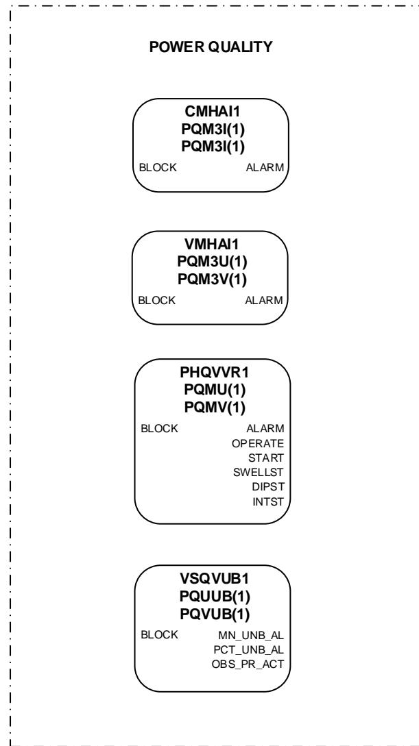
*Figure 41: Power quality measurement function*
