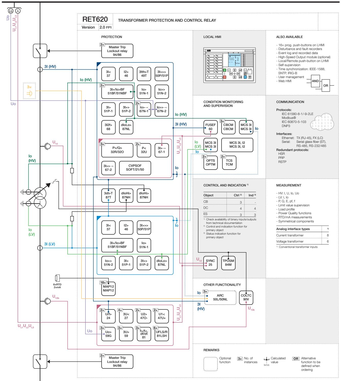
Figure 17: Functionality overview of default configuration with conventional instrument transformer inputs
