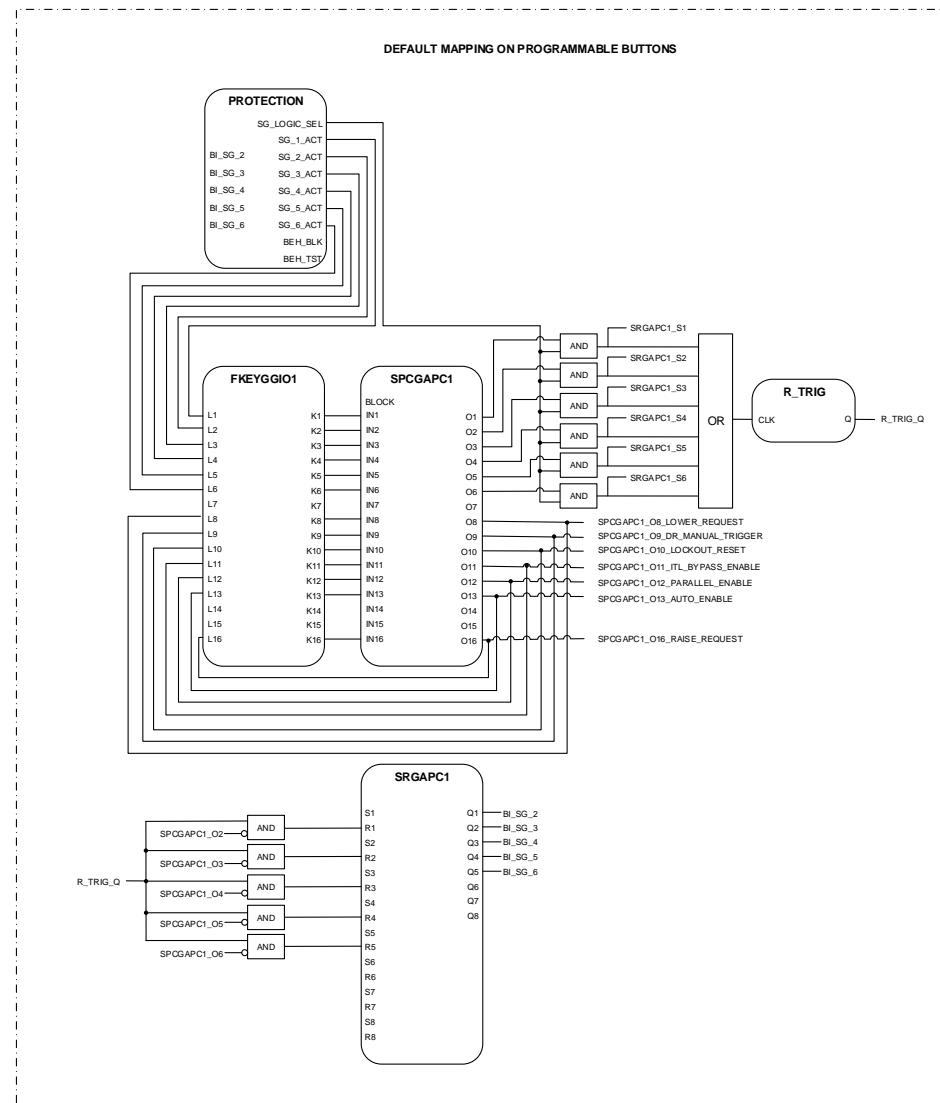
Figure 19: Default mapping on programmable buttons
