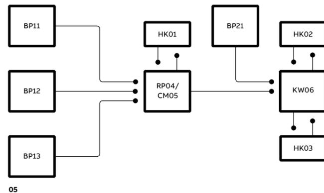
The modules are connected as shown in →5. Three of the feeder modules represent a dosing system for the mixing reactor. The mixing reactor feeds its product into a distillation stage that is also connected to a feeder module.
