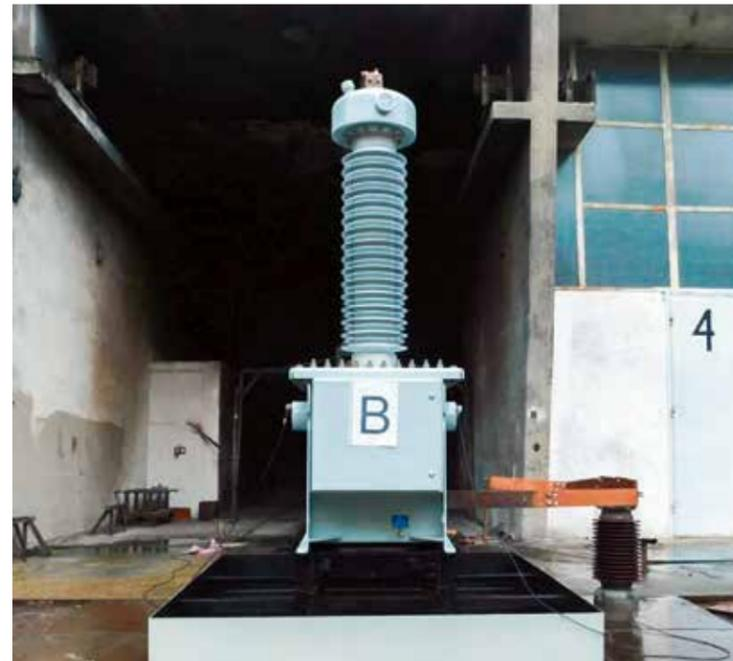
05 330 kV transformer tank pressure test.
