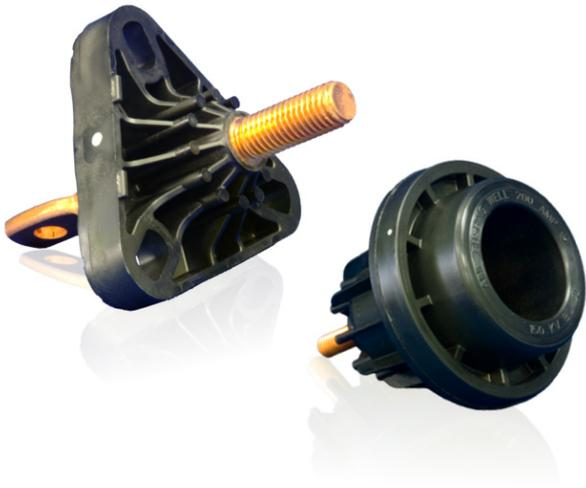
ABB offers both high voltage and low voltage bushings designed for use in pad or surface mounted transformers. The bushings insulate the current carrying conductor from the tank, allowing for termination of both the airside conductor and the transformer leads. Both the high and low voltage bushings have been designed to conform with ANSI/IEEE standards.
