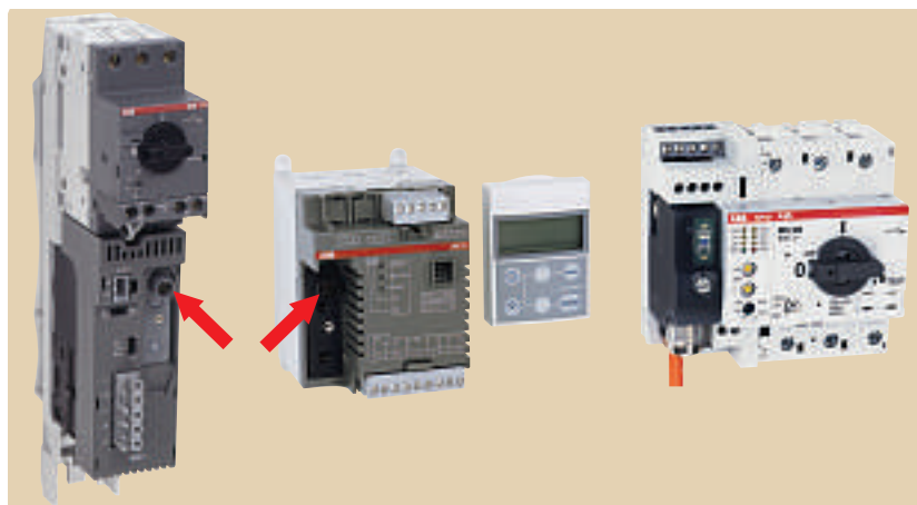
ABB starters so far equipped for the FieldBusPlug are the MSD11-FBP (far left), MSR22-FBP (not shown), both of which use MS 116, the UMC22-FBP (second from left) and the MFI21-FBP (right, with FBP installed), seen here connected to an MS 325. The arrows show the location of the FBP interface.
