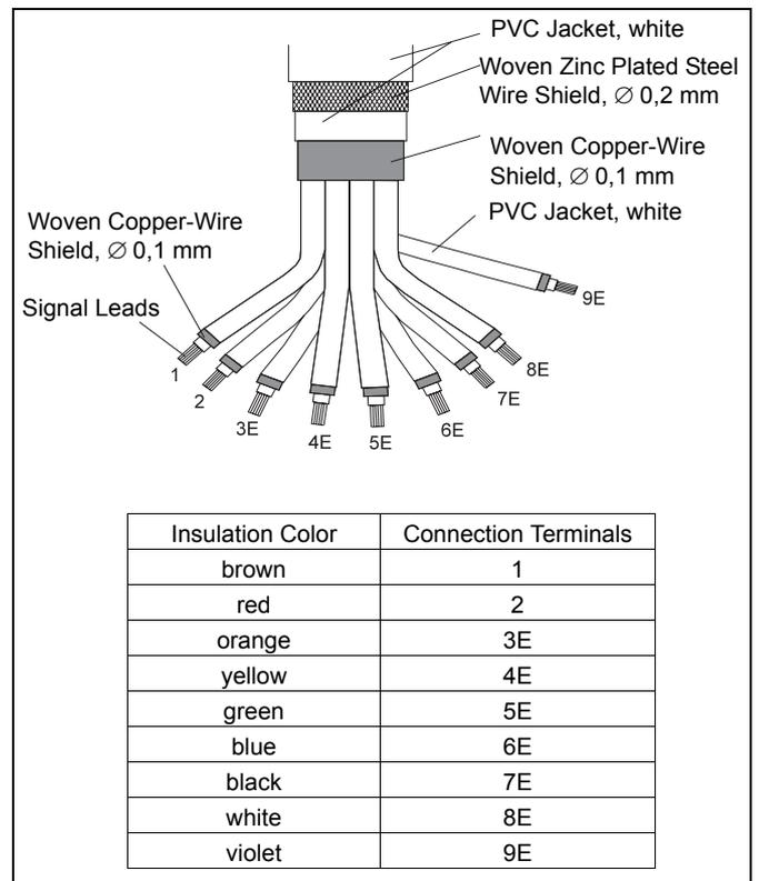
Fig. 33 Signal Cable Construction D173D021U01
