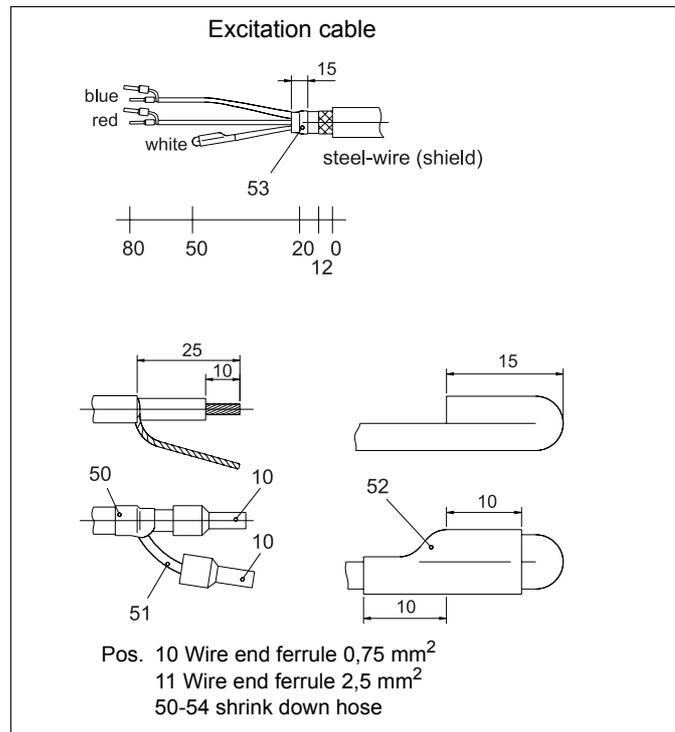
Fig. 36 Insulation of excitation cables
