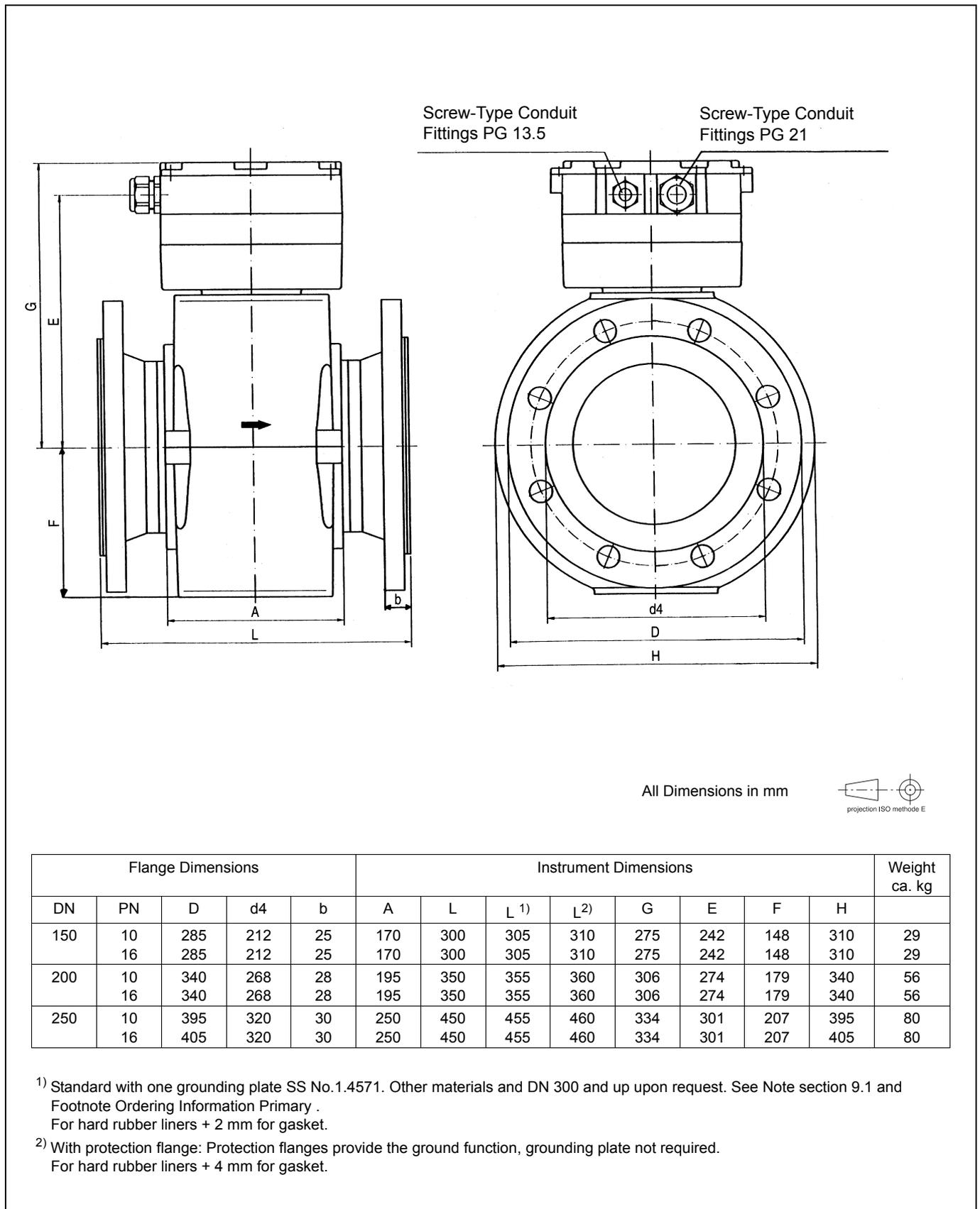
Fig. 22 Flowmeter Primary DN 150 to DN 250
