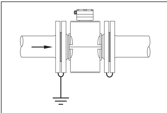
Fig. 27 Flowmeter Primary Meter Sizes 150 to 250, Two Piece Housing with Flanges
