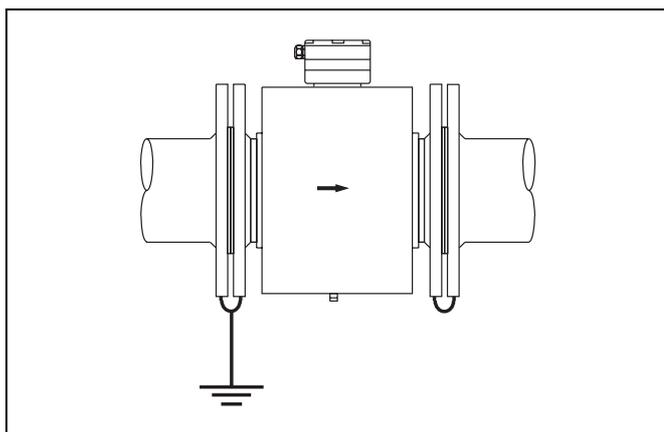
Fig. 31 Meter with an Integrated Conductive Element in the Liner
