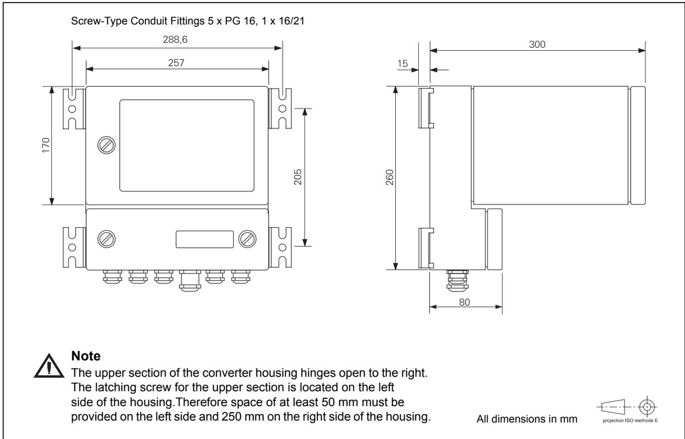
Fig. 25 Dimension Drawing, Field Mount Housing Converter MAG-XP
