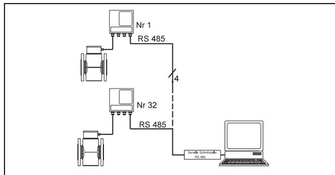
Fig. 48 Communication over Data Link RS 485
