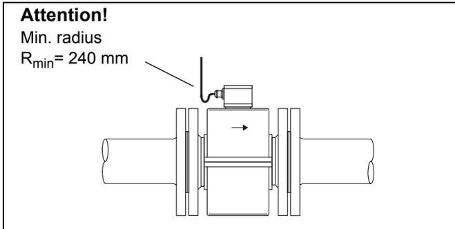
Fig. 37 Cable routing
