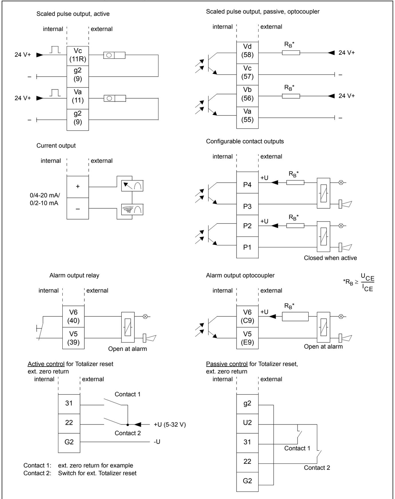
Fig. 46 Interconnection Examples for Peripherals
