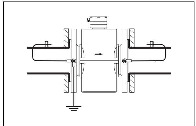
Fig. 29 Flowmeter Primary Meter Size 150 to 250 Two Piece Housing with Flanges
