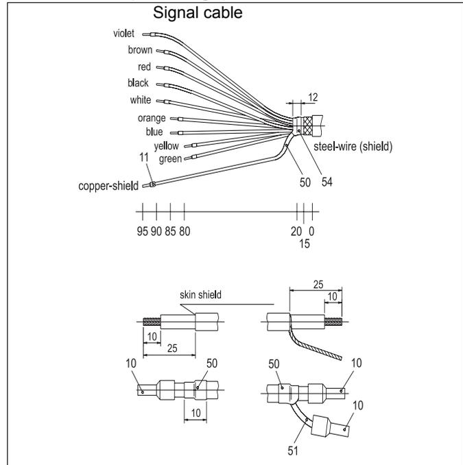
Fig. 35 Insulation of signal cables
