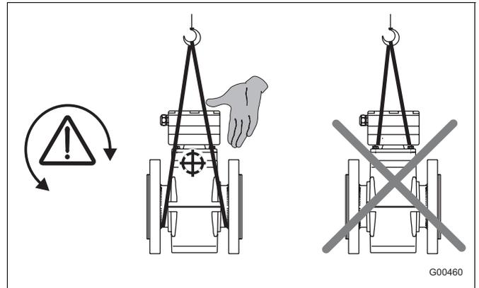
Fig. 2 Transport of flanged units < DN 300
