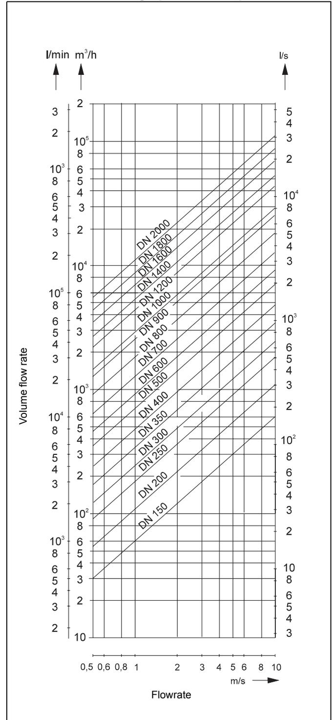
Fig. 12 Flow rate nomograph DN 150 - DN 2000
