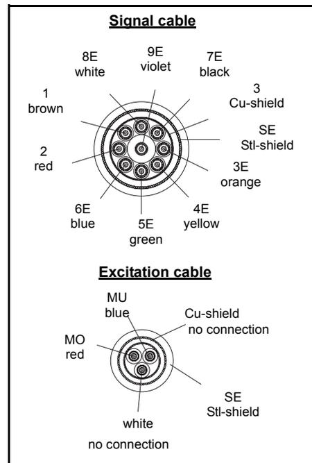
Fig. 44 Signal- and Coil Excitation Cable Connections
