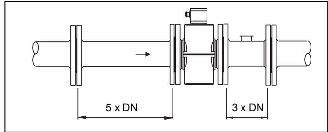
Fig. 5 In- and Outlet Sections
