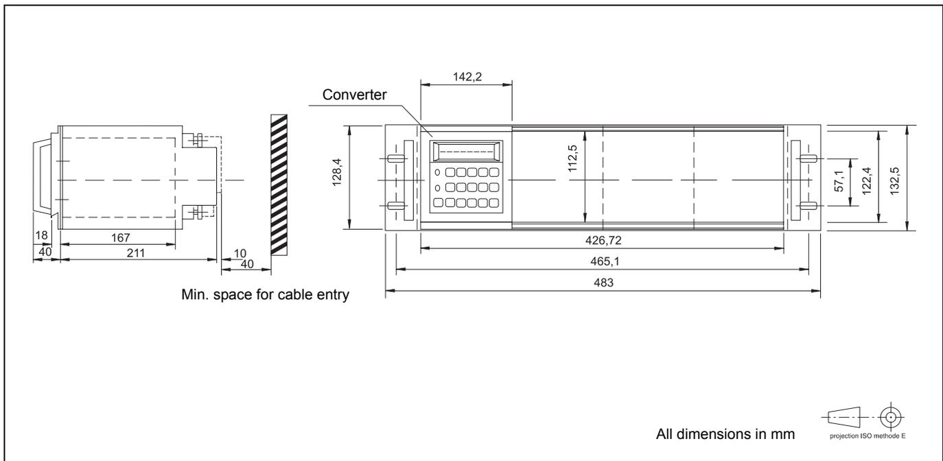
Fig. 26 Dimension Drawing, 19" Rack Mount
