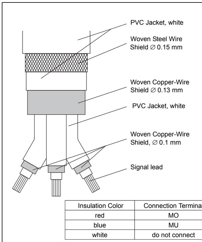
Fig. 32 Excitation Cable Construction D173D025U01
