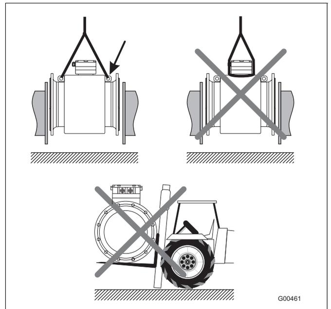
Fig. 3 Transport of flanged units > DN 250
