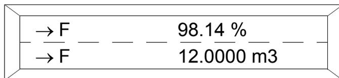
The totalizer value for the present flow direction is displayed in the second line with a maximum of 7 digits followed by the corresponding units. The totalizer value represents the actually measured flow volume independent of the pulse factor settings. This display configuration is designated as "Process Information" in the following text.
