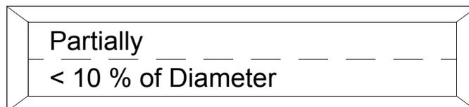
When the fill height drops below 10% of the flowmeter primary diameter the output signals are automatically turned off and a corresponding error message is displayed on the converter. The output signals are turned off when the fill height is less than 15 % in meter size 150 only.
