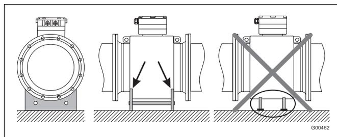
Fig. 7 Transport of flanged units > DN 300
