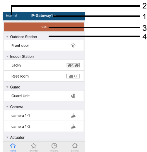
Figure. 38: After pairing the mobile APP with IP-Gateway, the APP will synchronize the lists from IP-Gateway automatically. All the devices should be set in IP-Gateway PC website in advance.
