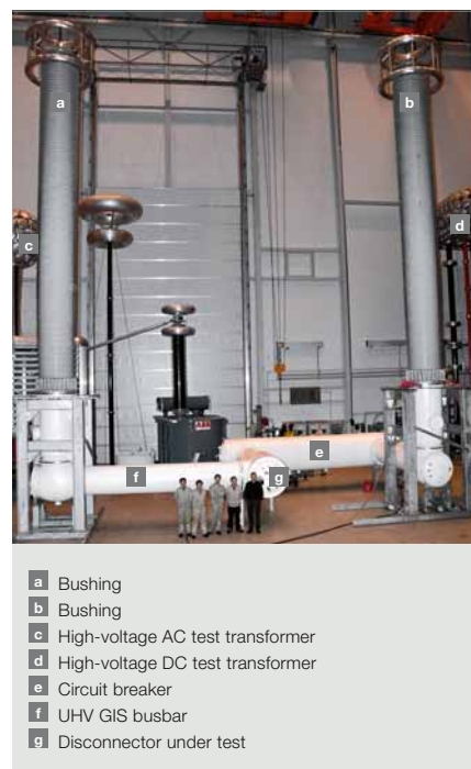
6 Arrangement for disconnecter switching tests at the STRI laboratory
