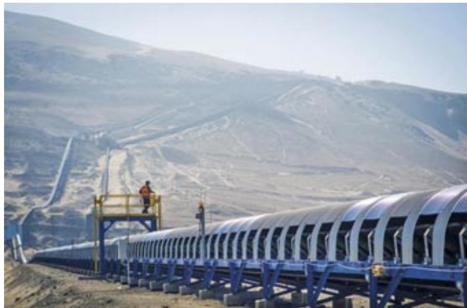
gearless motors; and an 1,830 mm wide, 1,043 m long overland conveyor #2 powered by head and tail end 550 kW VFD driven motors. Siemens supplied the complete electrical solution to thyssenkrupp. The EP project was awarded in 2014 and began operations in late 2017. Elsewhere on the current projects, for Oyu Tolgoi Siemens is supplying the gearless drives for the underground conveyor that feed a mine hoist (Phase 1) and the three incline conveyors for Phase 2.
