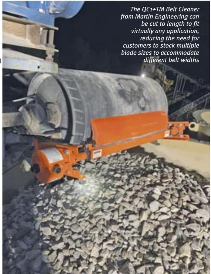
*The QC1+TM Belt Cleaner from Martin Engineering can be cut to length to fit virtually any application, reducing the need for customers to stock multiple blade sizes to accommodate different belt widths*
