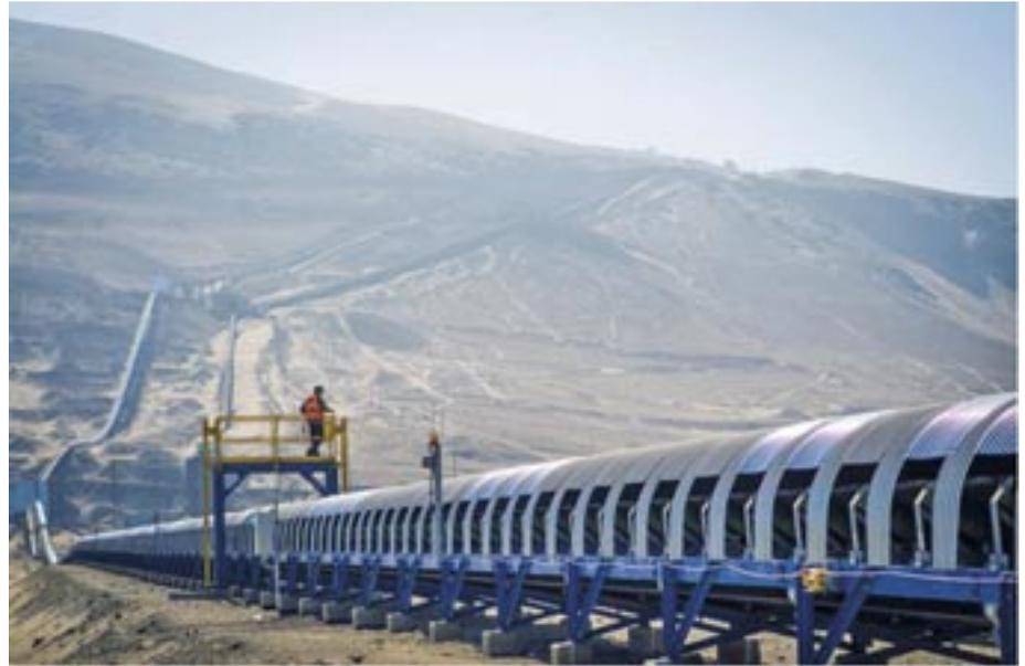
gearless motors; and an 1,830 mm wide, 1,043 m long overland conveyor #2 powered by head and tail end 550 kW VFD driven motors. Siemens supplied the complete electrical solution to thyssenkrupp. The EP project was awarded in 2014 and began operations in late 2017. Elsewhere on the current projects, for Oyu Tolgoi Siemens is supplying the gearless drives for the underground conveyor that feed a mine hoist (Phase 1) and the three incline conveyors for Phase 2.
