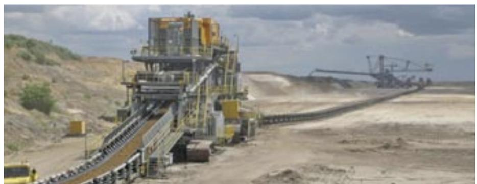
*Thanks to recent developments in condition and online monitoring of equipment and processes, availability will be increased as a result of ‘on demand’ planning for maintenance and service activities. Tenova TAKRAF has installed such systems on key equipment, in coordination with some of its end users*
