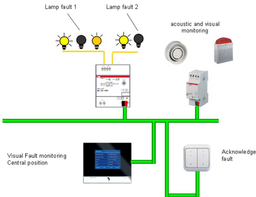
Fig. 35 System representation of a fault signal
