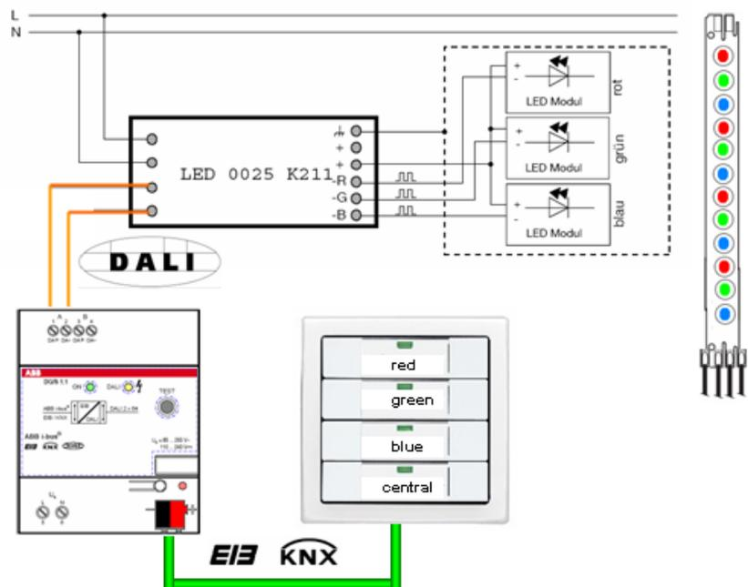
Fig. 25 Example of a colour LED system
