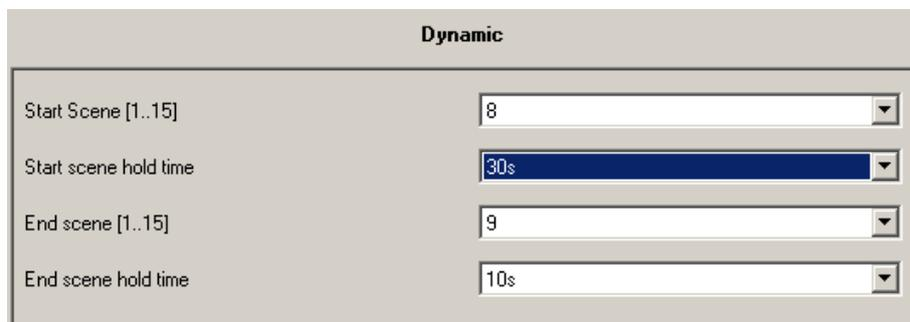
Fig. 29 Staircase lighting – Select start and end scene
