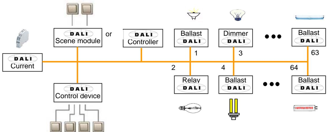
Fig. 1 DALI block diagram
