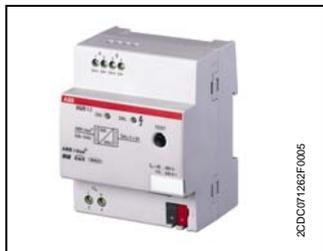
The 1-fold EIB/DALI-Gateway DG/S 1.1 is a modular installation device in *proM* design for installation in the distribution board on 35 mm mounting rails. The connection to the ABB i-bus® EIB / KNX is implemented via bus connecting terminals. The DALI-Gateway can integrate devices with a DALI interface into an EIB / KNX building installation using the application program "*Dim Lightscenes Dynamic 1f/x*".
