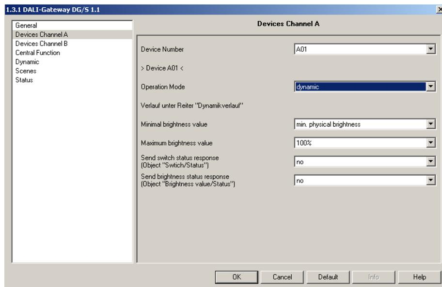
Fig. 9: Parameter window "Device – dynamic operating mode"
