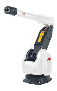
IRB 580 combines the advanced functions of the IRB 5400 series with a compact design. The result is a highly flexible, cost-effective and accurate paint robot system.
