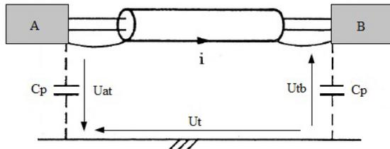
Figure 9: common mode disturbance circuit
