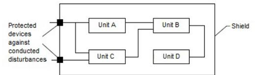
Figure 40: global protection system with single barrier
