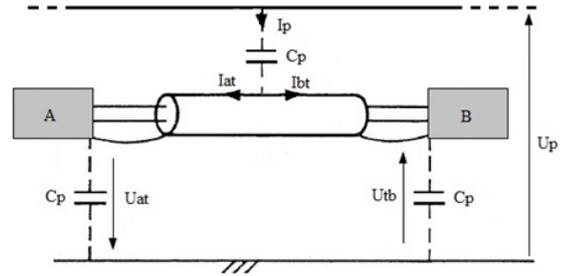
Figure 11: capacitive coupling circuit
