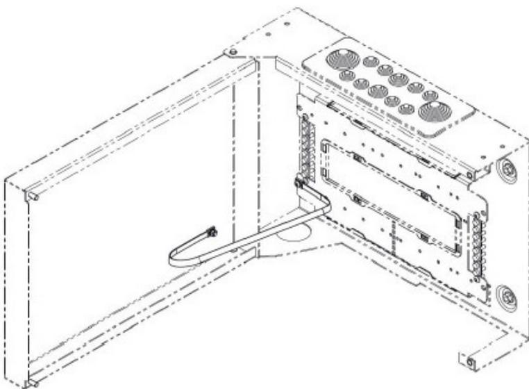
Figure 46: example of a connection between LV compartment and door
