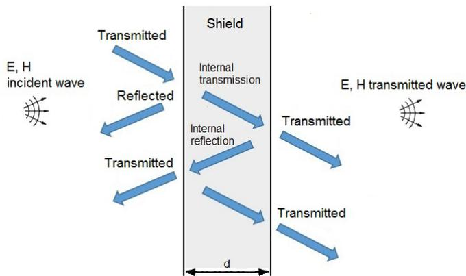
Figure 43: transmission of electromagnetic disturbances in a shield
