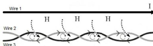
Figure 58: coupling diagram for twisted pair cable
