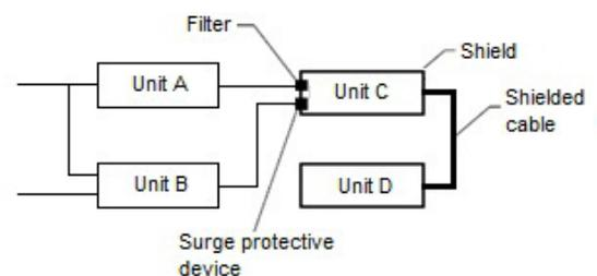
Figure 42: distributed protection system
