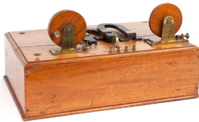
Figure 1: Original prototype of the radio wave detector that Guglielmo Marconi used in 1902 on board the cruiser Carlo Alberto.
