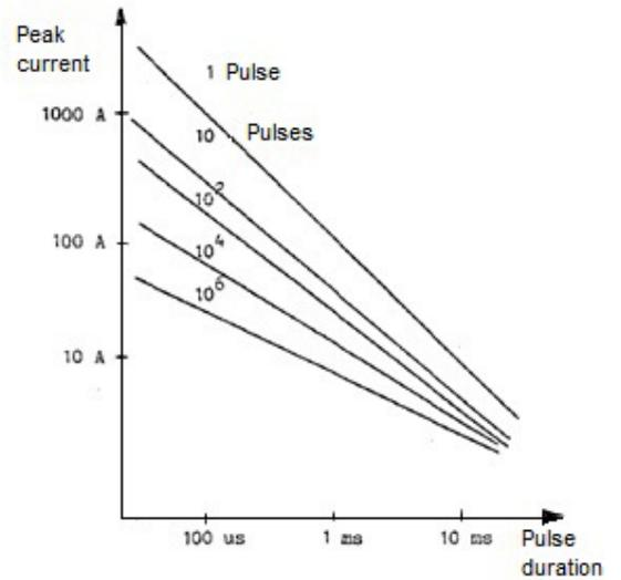
Figure 37: curves of the current peak supported by a varistor
