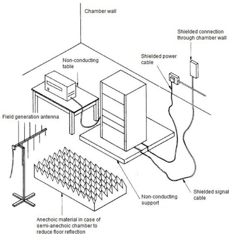
Figure 17: example with semi-anechoic chamber
