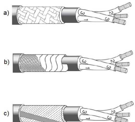
Figure 60: shield in conductive mesh a), with wound conductor b), wrapped in a helical fashion c)
