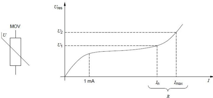
Figure 36: typical curve of a zinc oxide varistor (MOV)
