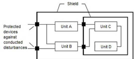
Figure 41: multiple barrier global protection system
