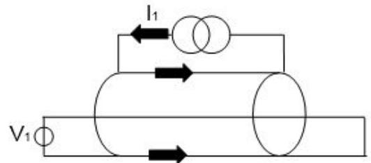
Figure 59: representative circuit for a shielded cable
