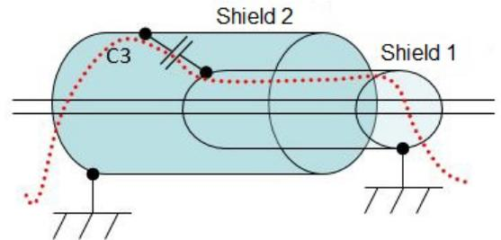
Figure 66: route taken by disturbance in a cable with double shield
