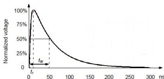
Figure 18: normalized waveform for EFT/BURST
