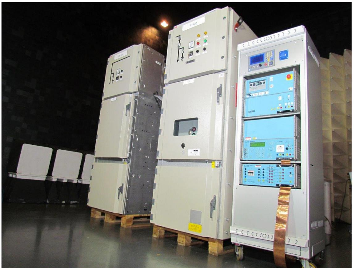
Figure 80: MV switchgear being tested in the ABB Dalmine EMC lab
