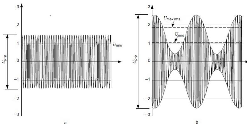
Figure 21: waveform of test level 1
