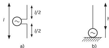
Figure 55: dipole antenna a) and monopole antenna b)
