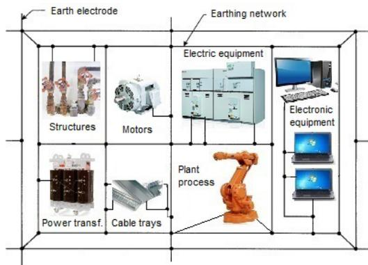
Figure 70: example of separation into zones in a building
