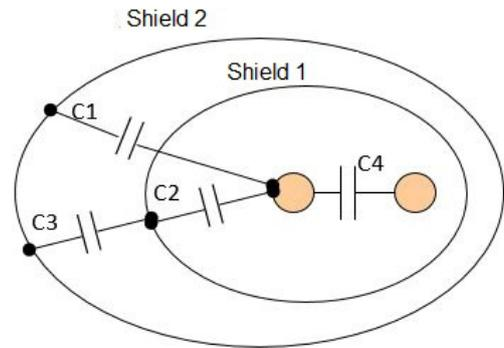
Figure 65: circuit of a cable with double shield
