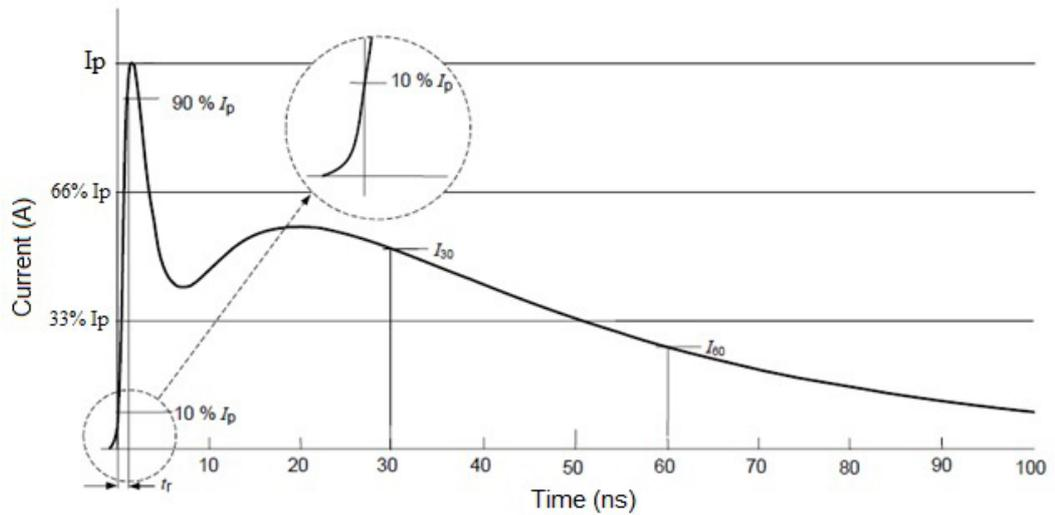
Figure 15: normalized waveform for ESD
