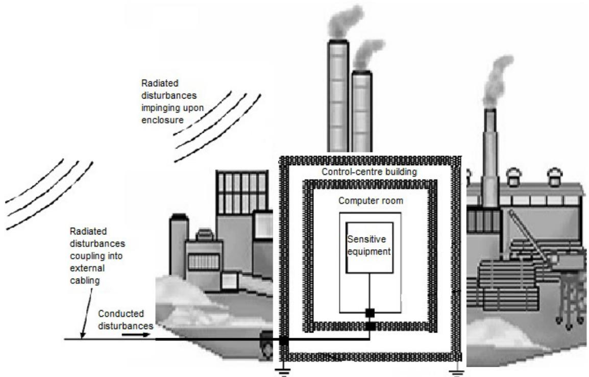
Figure 28: EMC for an industrial control center
