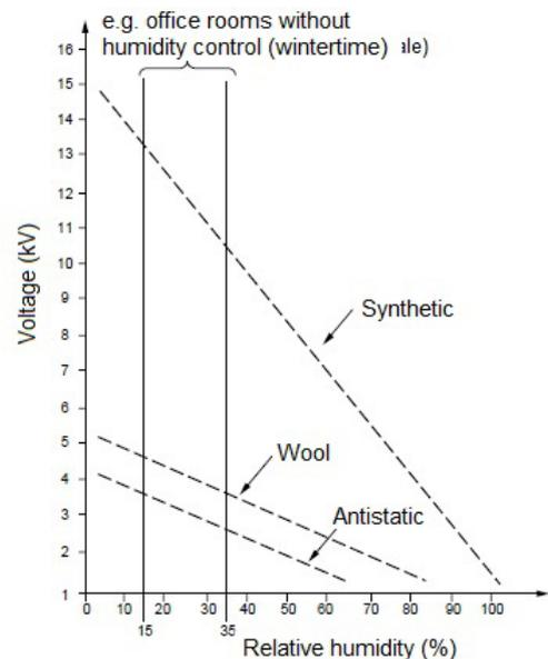
Figure 14: typical electrostatic discharge levels
