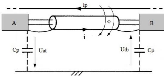
Figure 10: inductive coupling circuit
