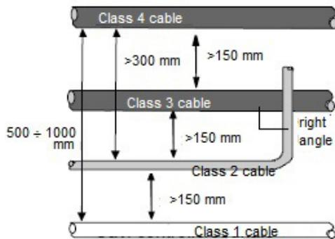
Figure 57: diagram of minimum distances between cables of different classes
