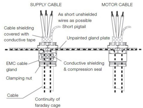
Figure 47: earthing with cable gland
