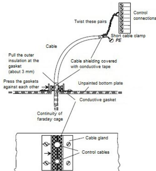
Figure 50: example of a correct connection
