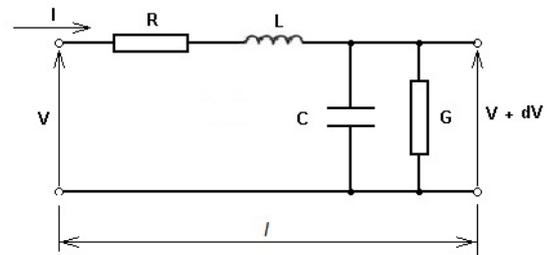
Figure 52: diagram of a conductor
