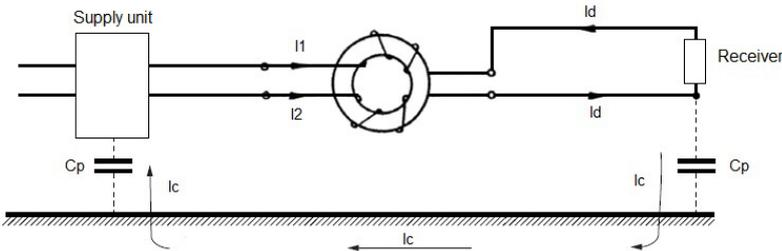
Figure 29: circuit with choke
