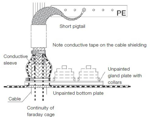
Figure 48: earthing with conductive sleeve
