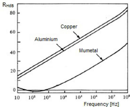
Figure 44: coefficient  $R_{HdB}$  in relation to frequency for certain materials
