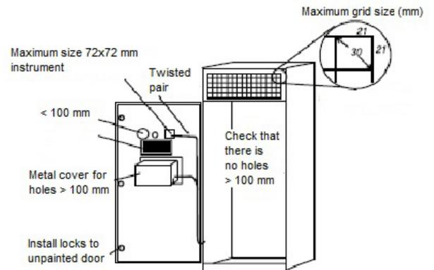
Figure 51: outline of EMC measures in a control panel
