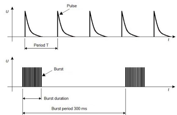
Figure 19: diagram of pulse burst
