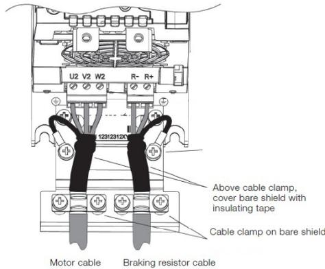
Figure 49: earthing with cable clamps
