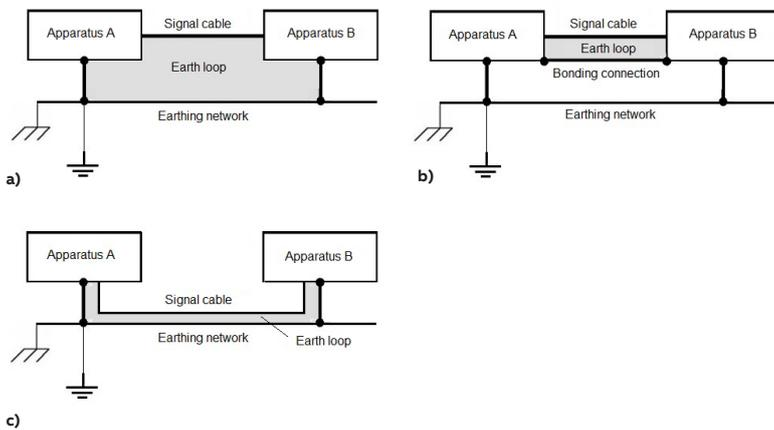
Figure 71: various ground loop configurations
