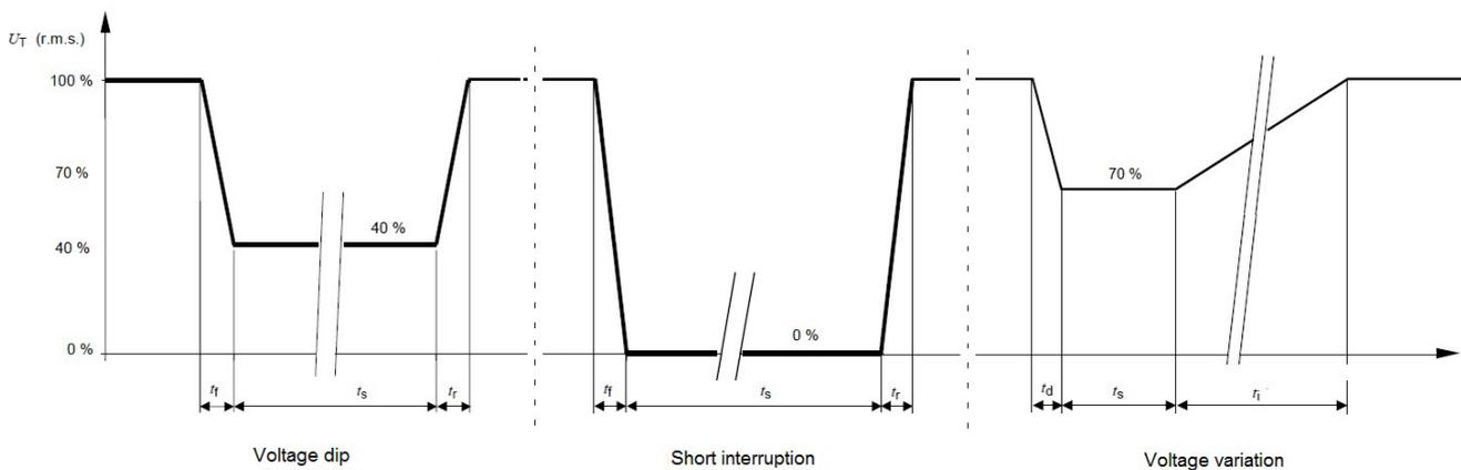
Figure 23: examples of voltage disturbance
