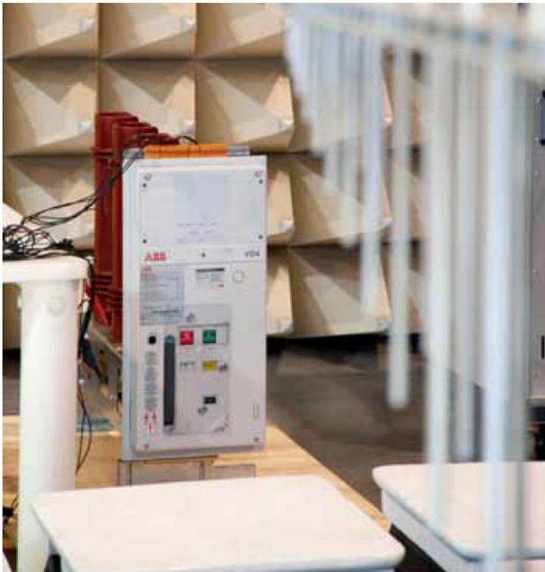
Figure 77: MV circuit breaker being tested in the anechoic chamber
