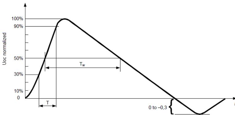
Figure 20: normalized waveform of a voltage surge
