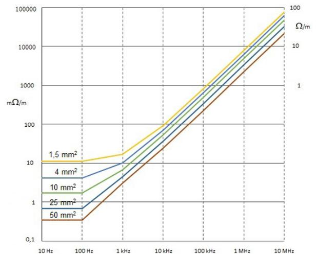
Figure 53: impedance in relation to frequency in certain cables
