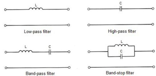
Figure 30: filters in series
