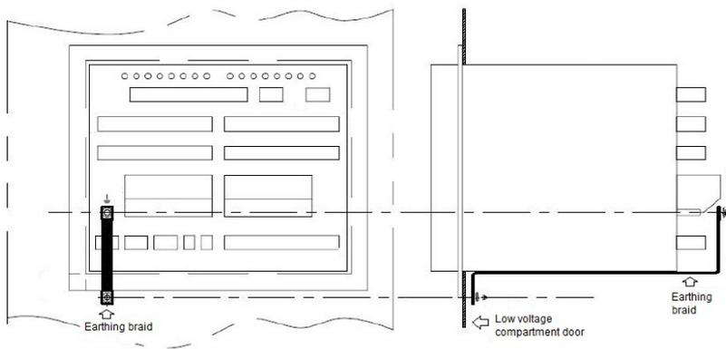
Figure 54: example of the earth connection of an IED
