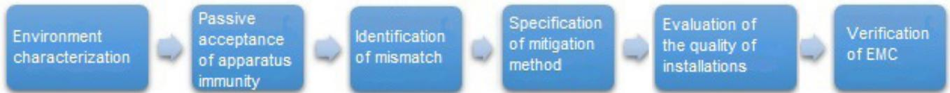
Figure 27: process to adopt for existing installations
