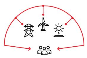
Conventional distribution networks feature a one-way power flow, where energy is drawn from high voltage power transmissions networks so as to supply the end users.
