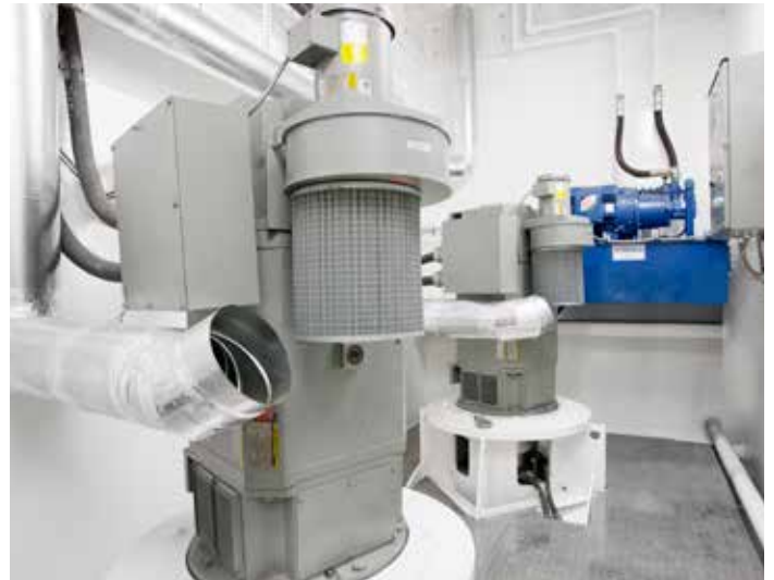
Drive controlled electric motors help reduce the thruster noise level.
