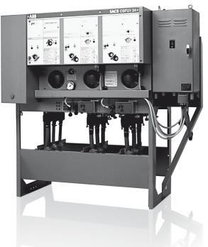
It was based on three positions line-open-earth disconnector units for the grid connection and the same device equipped with protection fuses for feeding power transformers. Both manually and electrically operated mechanisms were available during its active life cycle but most of them were delivered in the manually operation version only.
