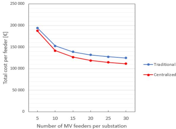
Fig. 4. The normalized total cost of the secondary system per MV feeder in traditional and centralized architectures for substations.
