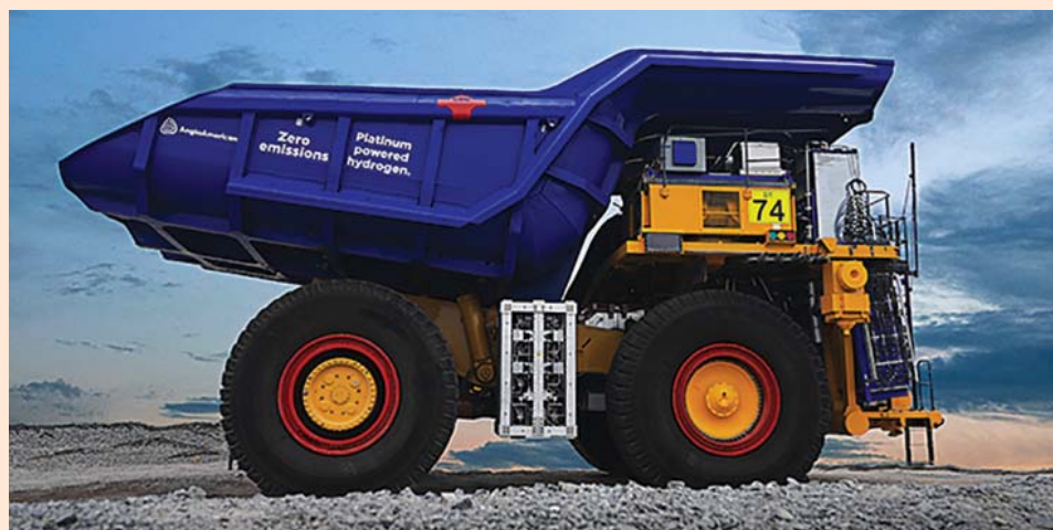
This is the first time a 290-mt haul truck has been converted to run on hydrogen. (Photo: Anglo American)
