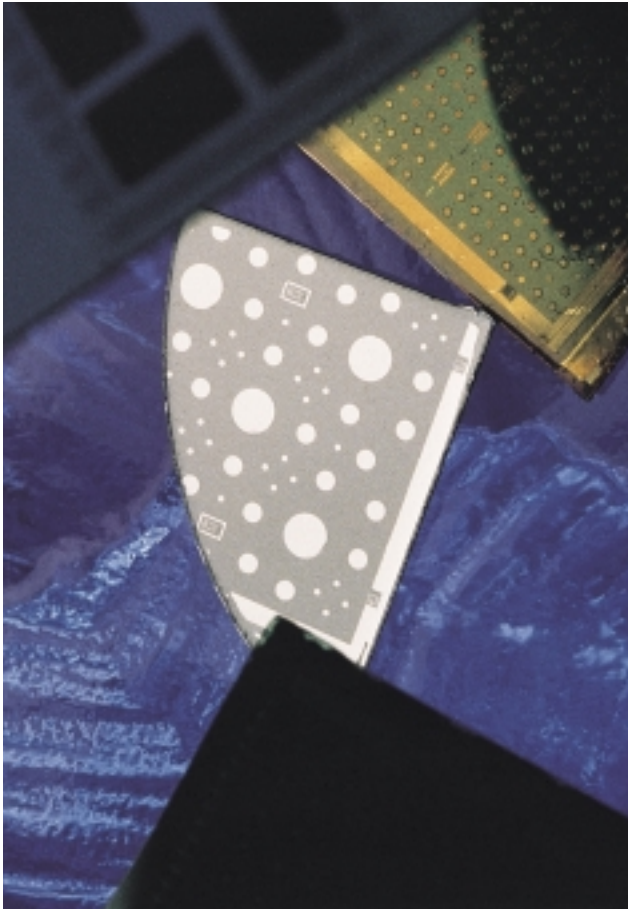
SiC test substrates (wafers) with diode structures of varying size
