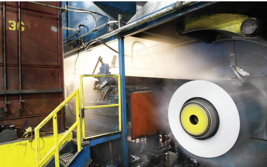
Jupiter Aluminum's three rolling mills are running with three Stressometer systems and six MTG thickness gauges.
