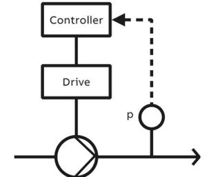
External signal to control the speed
