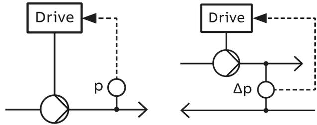
Outlet pressure or differential pressure as feedback to the drive to control the speed of the drive
