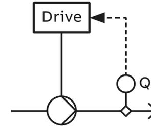
Flow as feedback to control the speed
