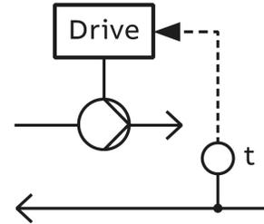
Temperature as feedback to control the speed
